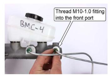
5. Thread the opposite end of the brake hard line installed in Step 4 into the front port of the stock proportioning valve.
