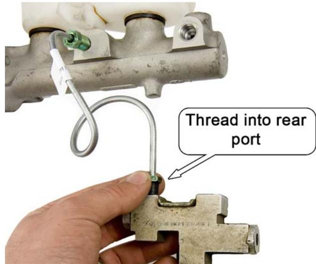
9. Thread the M10-1.0 bubble flare end of the "Forward Port" labeled brake hard line into the front port of the master cylinder. Position the free end of the hard line above the stock proportioning valve.
