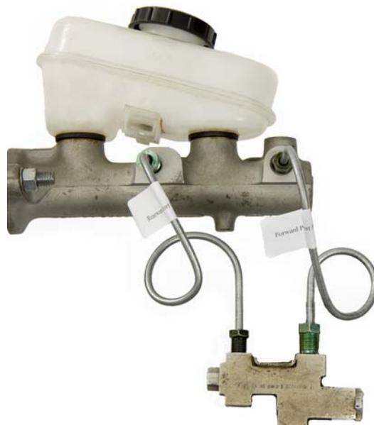
11. Tighten the ends of the brake hard lines to 12-16 ft-lbs at the master cylinder and the proportioning valve.
