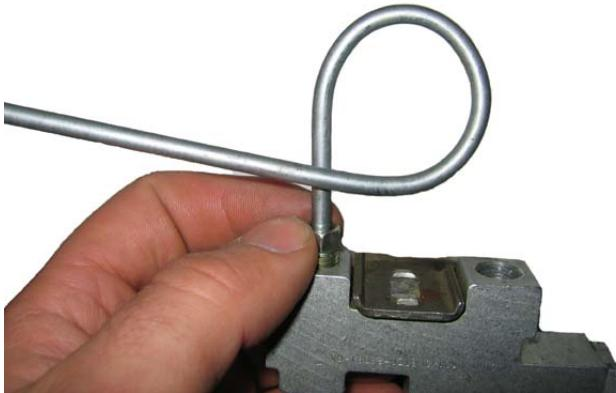
5. Thread the M10-1.0 bubble flare end of the "Forward Port" labeled brake hard line into the front port of the master cylinder. Position the free end of the hard line above the stock proportioning valve.
