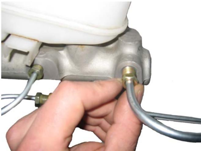
6. Thread the free end of the brake hard line into the front port of the stock proportioning valve.
