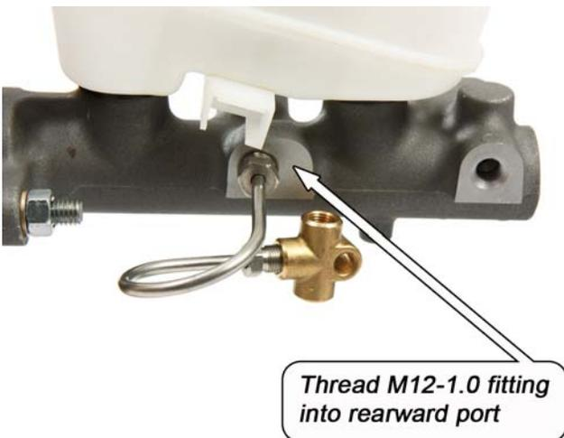
8. Attach the OEM brake line that was connected to the bottom of the old master cylinder to the bottom port of the Tee fitting. Only make the connection finger tight at this time.
