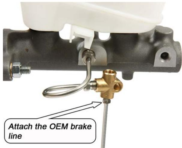
9. Thread the M10-1.0 end of the M10-1.0 to 3/8-24 brake hard line into the remaining port on the Tee fitting, and thread the free end into the rearward port of the stock proportioning valve.
