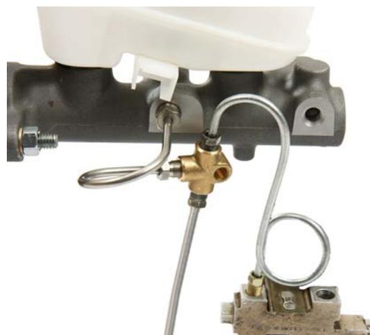
10. Thread the M10-1.0 bubble flare end of the "Forward Port" labeled brake hard line into the front port of the master cylinder. Position the free end of the hard line above the forward port of the stock proportioning valve.
