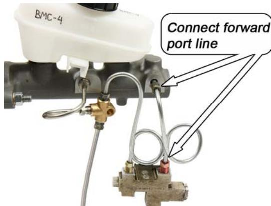
12. Tighten the ends of the brake hard lines to 12-16 ft-lbs at the master cylinder and the proportioning valve.
