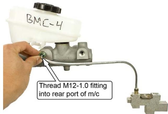
3. Thread the free end of the brake hard line installed in Step 2 into the rear port of the stock proportioning valve (3/8-24 fitting).
