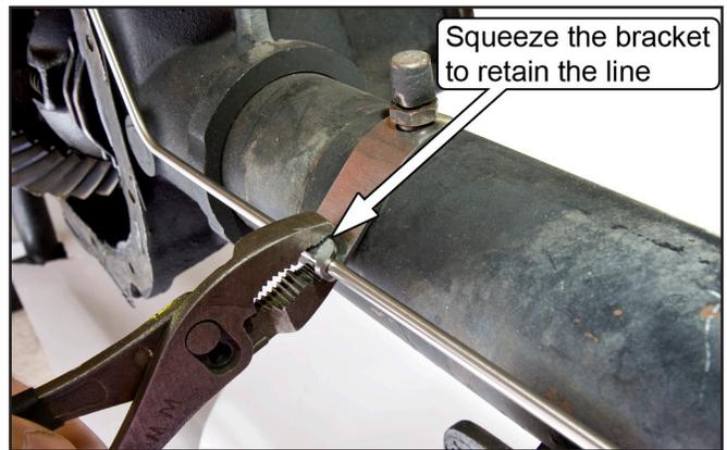
23. Tighten the Axle Vent fitting while holding the Brake Hard Line Mounting Bracket.
