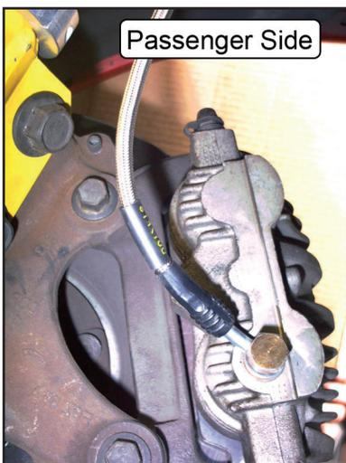
12. Torque the fluid bolt at the caliper to 14 ft-lb while holding the black plastic strain relief of the hose to keep the hose from rotating.
