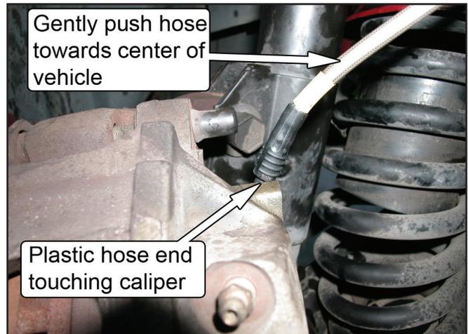
11. Torque the fluid bolt at the caliper to 14 ft-lb while gently pushing the brake hose toward the center of the car with two fingers to keep it from rotating.
