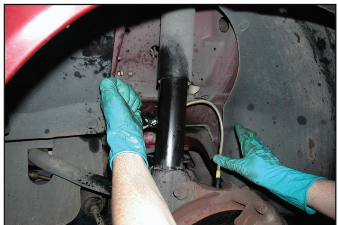
13. Temporarily remount the wheels; checking clearances to ensure the hose will not contact the tire. Have a helper turn the steering wheel from lock to lock. If it does rub, the tire *will* wear through the hose.
