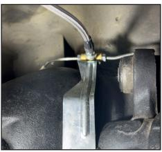
13. Attach the banjo fitting to the chassis hardline fitting by using the supplied fluid bolt and 2 new copper washers.
