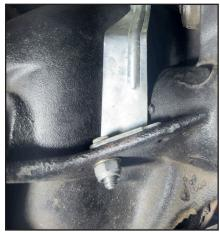
12. Attach the two axle hardlines to the T-fitting. Take care to avoid cross-threading the tube nuts. Tighten the tube nuts.
