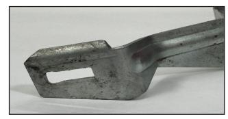
8. Attach the MM rear hose assembly to the bracket. Pass the 1/4" bolt upward through the enlarged slot and through the MM hose T-fitting. Place the supplied flat washer on the bolt and secure with the 1/4" locking nut. Orient the T-fitting lengthwise, as was the stock T-fitting.
