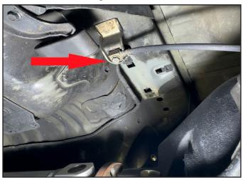
5. Remove the mounting bracket from the rear axle housing by removing the retaining nut.
