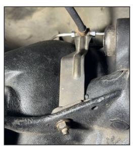
The differential mounting bracket will be reused with the MM hose. Simply cut, grind, or file off the tab which protrudes through the bracket from the 'T' fitting. That allows separating the factory hose/T-fitting assembly from the bracket.
