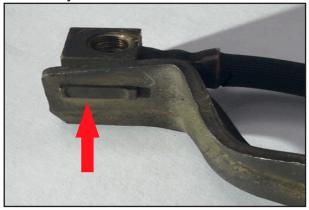
7. Drill or file a hole at the end of the slot in the bracket large enough for the supplied 1/4" bolt to pass through the slot. This should be at the end of the slot closest to the edge of the metal bracket.
