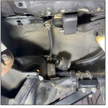
3. Remove the two hardlines from the T-fitting on the axle. Use a flare-nut wrench to avoid rounding off the tube nuts.
