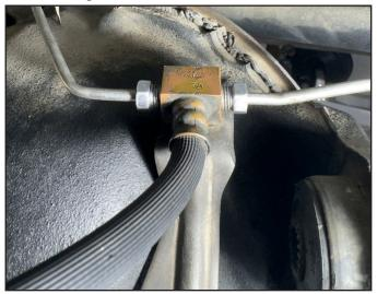
4. Remove the fluid bolt securing the hose to the chassis fitting.
