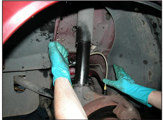
14. Secure the hose end to the chassis bracket by re-using the factory 'C-clip'.
