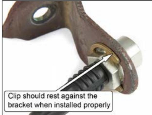
*NOTE: For 1979-86 and 1987-93 4 cylinder vehicles, the hole in the bracket must be enlarged to accommodate the brake hose.*
