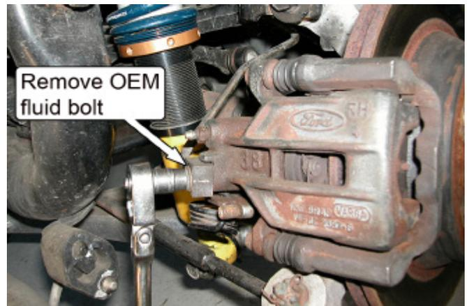
Remove OEM fluid bolt
