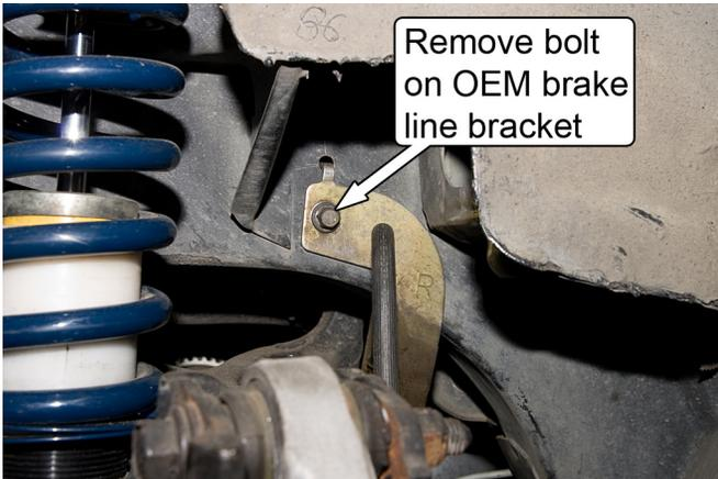
Remove bolt on OEM brake line bracket
