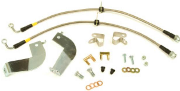
These Maximum Motorsports DOT approved braided stainless steel Teflon-lined brake hoses surpass the quality, fit, and finish of anything else in the Mustang aftermarket industry. These hoses provide better performance because their Teflon lining does not expand under pressure like a typical rubber line will. Installing stainless steel hoses will provide quicker braking response, improved modulation and a firmer brake pedal.
