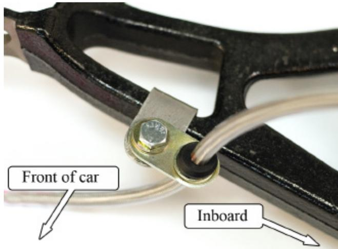
12. Bolt the metal brake hose mount (preinstalled on the brake hose) to the top side of the MM IRS Control Arm Bracket on the control arm. Use a supplied 1/4" G5 hex bolt, two (2) G8 washers and a G8 nylock nut to secure the brake line. Tighten the bolt until the brake hose mount cannot move.
