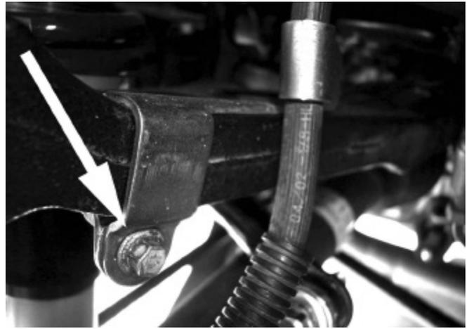
6. Disconnect the OEM brake hose from the brake caliper. Use a 10mm wrench or socket to remove the stock fluid bolt.
