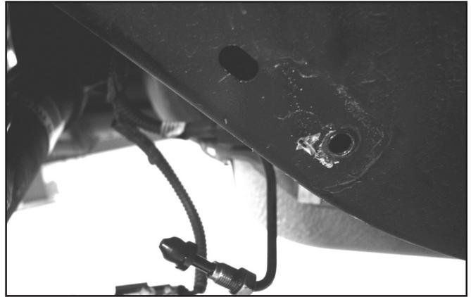
7. The supplied driver and passenger side mounting brackets are identical. Orient a mounting bracket to the frame rail just as the stock bracket was, and attach using the factory bolt.
