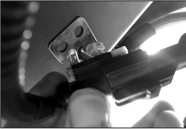
4. Disconnect the hard line. Use a flare nut wrench to avoid rounding off the fitting.
