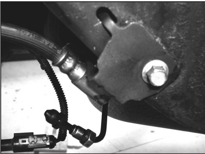
5. Disconnect the fluid bolt at the brake caliper.
