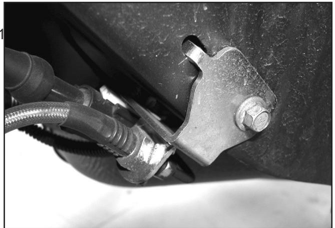
9. Place one crush washer under the head of one of the supplied fluid bolts. Pass the bolt through the MM brake hose. Place a second crush washer over the bolt so that the brake line fitting is sandwiched between the two crush washers.
