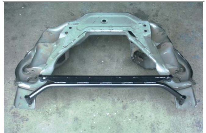
4-Point K-Brace placement on the K-member as viewed from the rear of the car
