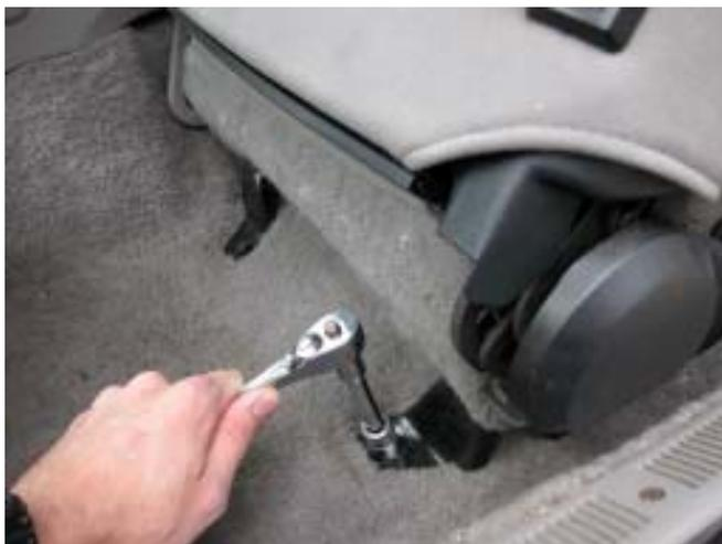
2. Install the supplied longer 10mm bolts with a washer under each head.
