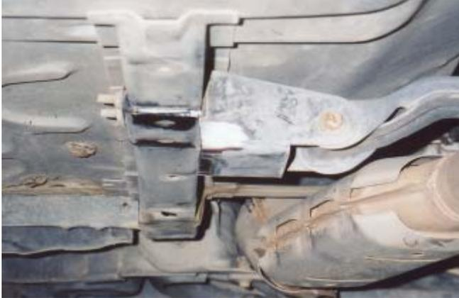
Weld transmission mount to subframe before installing subframe connector
