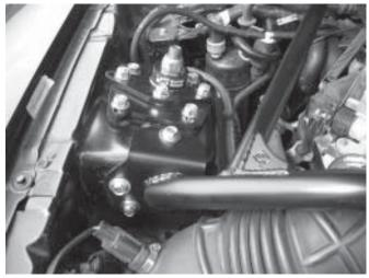
5. Start the bolts at the firewall mount with the 8mm large diameter washers.
