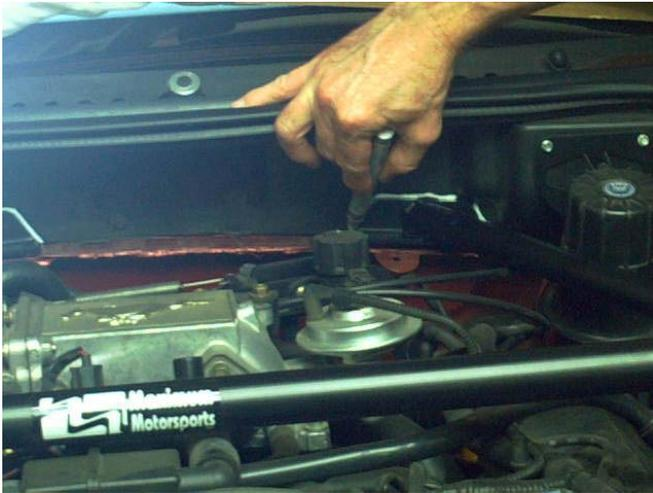
7. Cut out the portion of the plastic you marked. *Tip:* use a hacksaw on the vertical cuts. Use a utility knife to score the plastic on the horizontal cut, then bend and break the plastic on the scored line.
