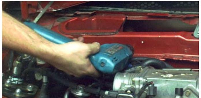
17. Drill the holes at the firewall. Start with a 1/8" pilot bit. Drill out to 5/16". deburr the holes. Note: Hold the hood vertical when drilling downwards into the pinchweld. That will provide clearance for the drill motor. *Tip:* Hold the hood upright by using a rope or strap to tie the hood to the steering wheel.
