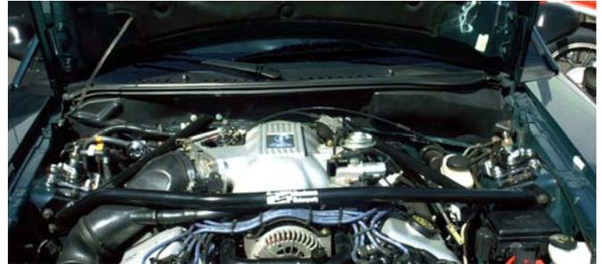
*NOTE:* Access to the fuse box -- the cover can still be opened by pulling the cover forward and past the strut brace main tube as you lift the cover.
