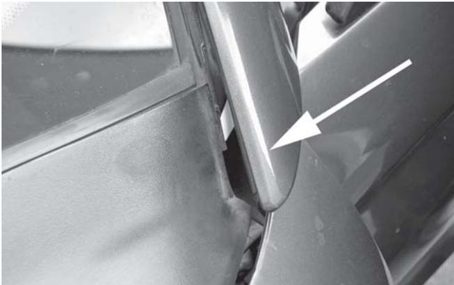
12. Remove the plastic cowl cover at the base of the windshield. It is held on with clips. Remove it by gently prying it upwards. When it is loose, disconnect the hose to the windshield washer nozzles (pointed to below).
