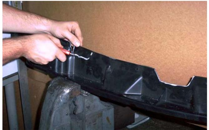
6. Remove the alarm siren (if so equipped) from the firewall. Then remove the plastic cover from the firewall. It is held on with several small sheet metal screws, as well as the hood seal.
