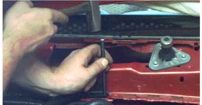
15. Remove the 6 bolts at the strut towers. Remove the Strut Tower Brace.
