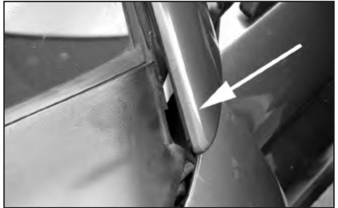
16. Remove the plastic cowl cover at the base of the windshield. It is held on with clips. Remove it by gently prying it upwards. When it is loose, disconnect the hose to the windshield washer nozzles (pointed to below).
