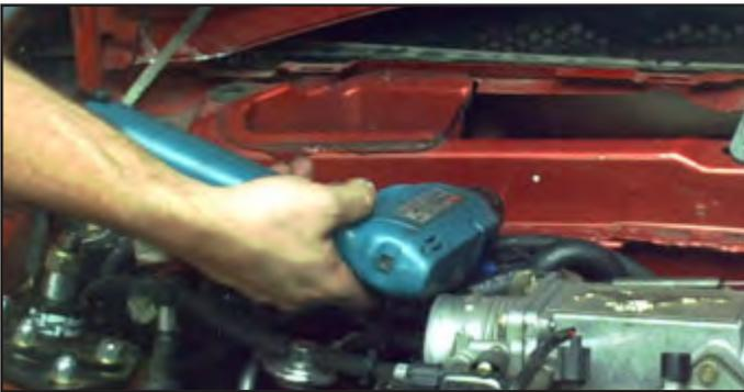
21. Drill the holes at the firewall. Start with a 1/8" pilot bit. Drill out to 5/16" and deburr the holes. Note: Hold the hood vertical when drilling downwards into the pinch weld. That will provide clearance for the drill motor. *Tip:* Hold the hood upright by using a rope or strap to tie the hood to the steering wheel.
