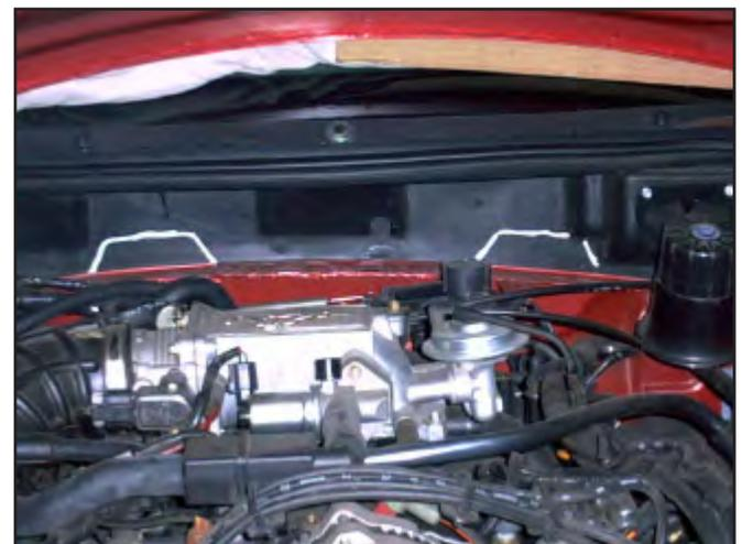
5. Remove the alarm siren (if so equipped) from the firewall. Then remove the plastic cover from the firewall. It is held on with several small sheet metal screws, as well as the hood seal.
