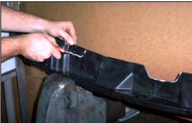
7. Put the plastic back into position on the firewall. Set the Strut Tower Brace back into position and check that the plastic is notched correctly.
