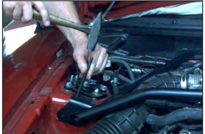
10. Center punch the mark. Drill a 1/8" pilot hole. Drill out to 5/16". Deburr the hole.
