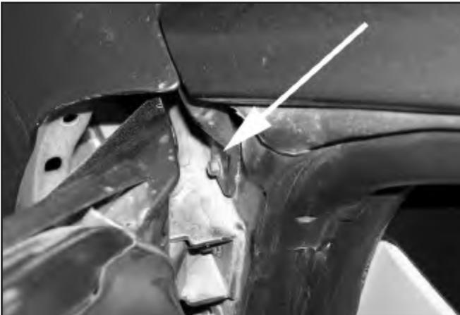
15. DO NOT remove the applique. Gently move it away just enough to open a small gap for removal of the plastic cowl at the base of the windshield.
