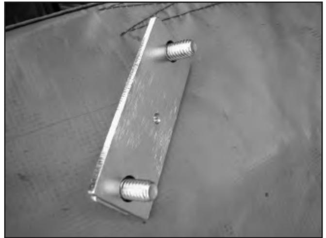
23. Line up the nut plate on the 5/16" holes drilled in the firewall in Step 20. Use the bolts installed in the previous step as guide pins. Make sure that the small hole in the plate is biased downward.
