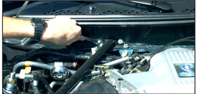
35. Tighten the bolts at the pinchweld.
