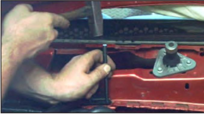
19. Remove the 6 bolts at the strut towers. Remove the Strut Tower Brace.
