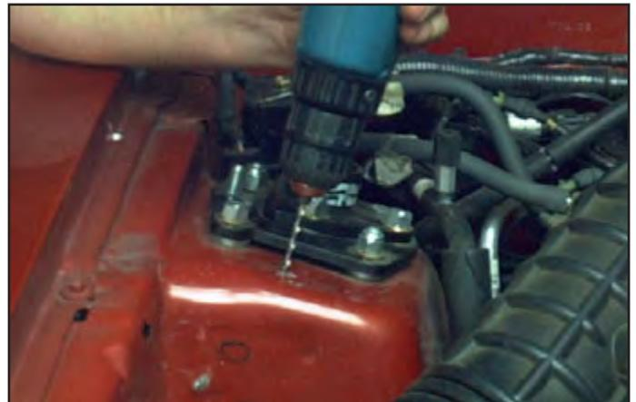
11. Set the Strut Tower Brace back into place. Insert a 5/16" bolt into the hole to hold the brace in position. Hold it both downwards and rearwards. Mark the positions of all of the other holes on both strut towers. Remove the Strut Tower Brace before drilling.
