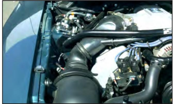
4. Mark the position of the strut tower brace on the plastic covering the firewall.
