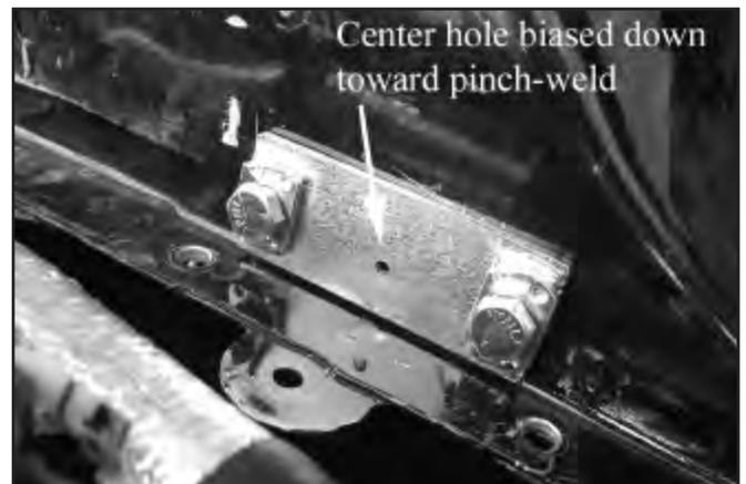
24. Using the nut plate as a template, mark the location of the small hole using a scribe or punch.
