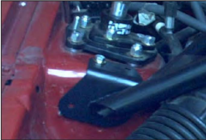
12. Center punch each mark. Drill a 1/8" pilot hole. Drill out to 5/16". Deburr the holes.
