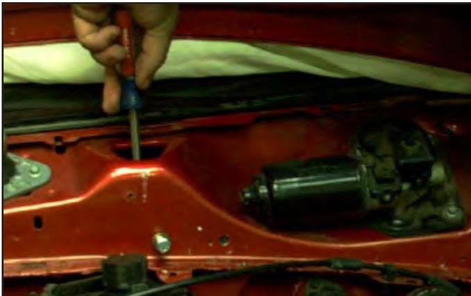
31. Install the #8 sheet metal screw into the small hole in the nut plate. Remove the 5/16"-18 bolts.
