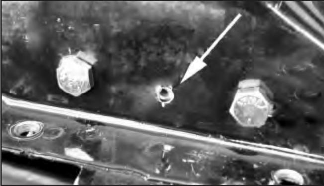
*Tip: On the Driver's Side, tape the nut plate to a screwdriver to help hold it in position behind the firewall while installing the bolts.*
