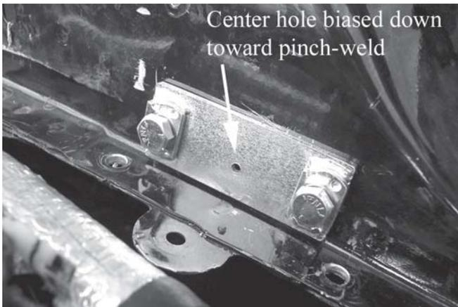
21. Using the nutplate as a template, mark the location of the small hole using a scribe or punch.
