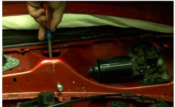
28. Install the #8 sheet metal screw into the small hole in the nutplate. Remove the 5/16"-18 bolts.
