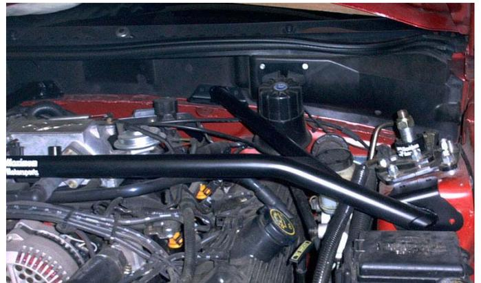
4. Bolt the Strut Tower Brace to the strut towers at the stock location. Use either the original Ford bolts, or the supplied 8mm bolts.
