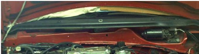
8. Cut out the portion of the plastic you marked. *Tip:* use a hacksaw on the vertical cuts. Use a utility knife to score the plastic on the horizontal cut, then bend and break the plastic on the scored line.
