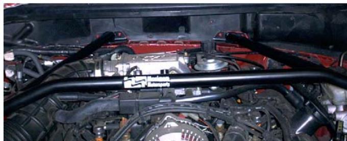
10. Remove the plastic cover from the firewall.
