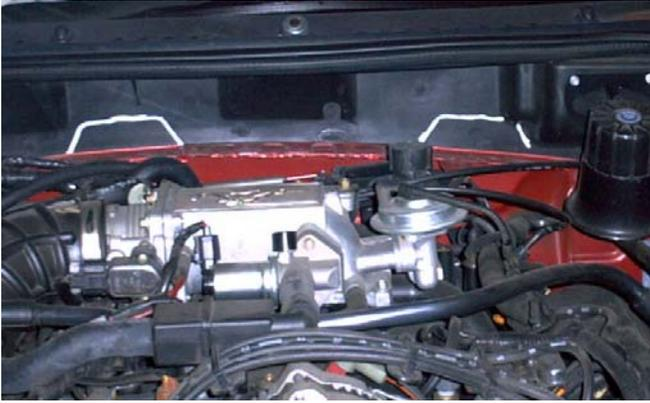
7. Remove the alarm siren (if so equipped) from the firewall. Remove the hood seal from the cowl. Then remove the plastic cover from the firewall. It is held on with several small sheet metal screws.
