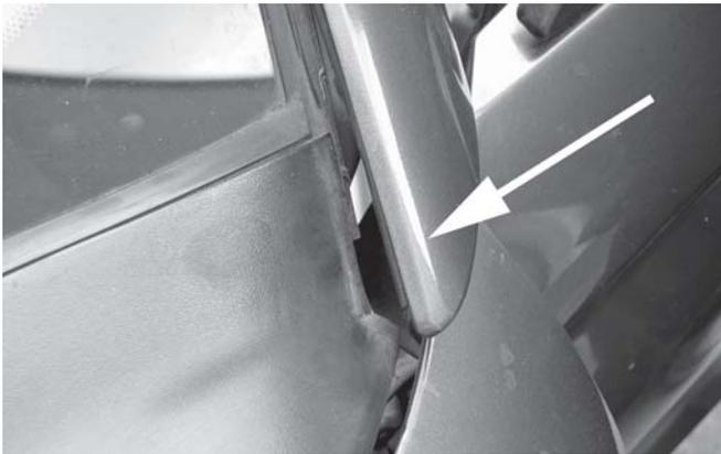
13. Remove the plastic cowl cover at the base of the windshield. It is held on with clips. Remove it by gently prying it upwards. When it is loose, disconnect the hose to the windshield washer nozzles (pointed to below).
