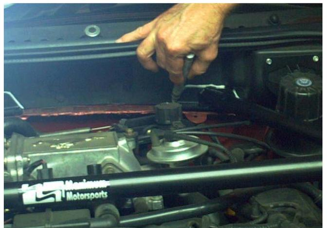
6. Remove the Strut Tower Brace.
