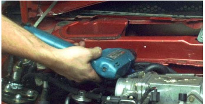
18. Drill the holes at the firewall. Start with a 1/8" pilot bit. Drill out to 5/16". Deburr the holes. Note: Remove the hood or hold it vertical when drilling downwards into the pinchweld. That will provide clearance for the drill motor. *Tip:* Hold the hood upright by using a rope or strap to tie the hood to the steering wheel.
