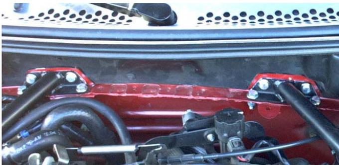
33. Tighten the bolts at the strut towers.
