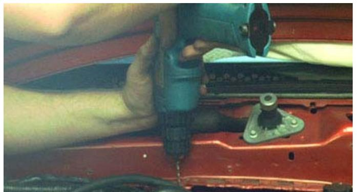
19. Install the 5/16"-18 x 3/4" long bolts in the nutplate. Thread them through so that they protrude on the flat side of the nutplate. It is not necessary to thread the bolts all the way in.
