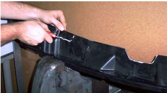
9. Put the plastic back into position on the firewall. Set the Strut Tower Brace back into position and check that the plastic is notched correctly.
