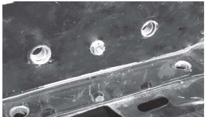
*NOTE:* This will secure the nutplate to the firewall, making future removal and reinstallation of the Strut Tower Brace significantly easier. The head of the sheet metal screw should line up with the hole at the back of the strut tower brace mounting pad.
