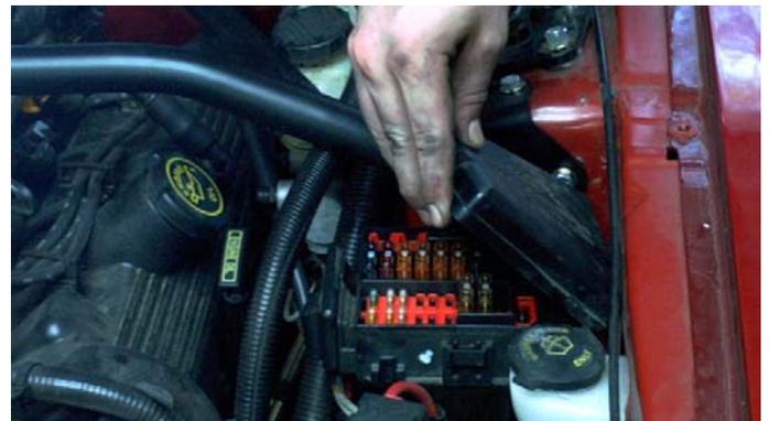
*NOTE: If the fuse box cover cannot be opened, reposition the fuse box by moving it forward. This can easily be done by slipping a screwdriver between the front of the strut tower and the rear of the metal fuse box mounting tabs (these are attached to the strut tower). Gently pry the tabs forward. This will move the fuse box slightly forward.*
