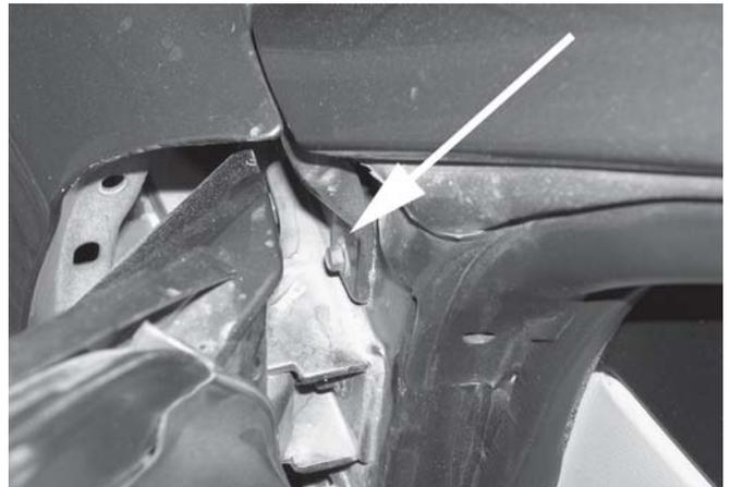
12. DO NOT remove the applique. Gently move it away just enough to open a small gap for removal of the plastic cowl at the base of the windshield.
