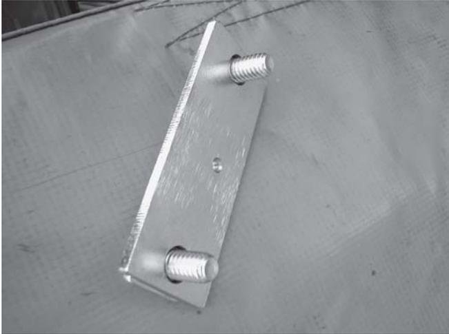
20. Line up the nutplate on the 5/16" holes drilled in the firewall in Step 19. Use the bolts installed in the previous step as guide pins. Make sure that the small hole in the plate is biased downward.
