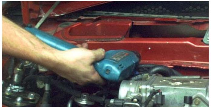
18. Drill the holes at the firewall. Start with a 1/8" pilot bit. Drill out to 5/16". Deburr the holes. Note: Remove the hood or hold it vertical when drilling downwards into the pinchweld. That will provide clearance for the drill motor. *Tip:* Hold the hood upright by using a rope or strap to tie the hood to the steering wheel.
