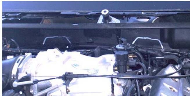
8. Remove the alarm siren (if so equipped) from the firewall. Remove the hood seal from the cowl. Then remove the plastic cover from the firewall. It is held on with several small sheet metal screws.
