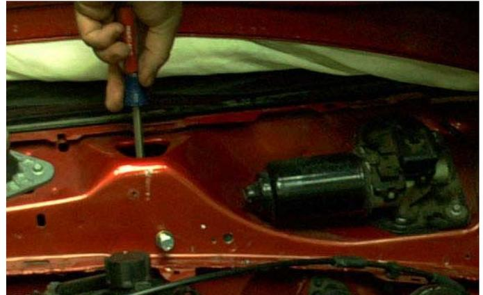
33. Install the #8 sheet metal screw into the small hole in the nutplate. Remove the 5/16"-18 bolts.
