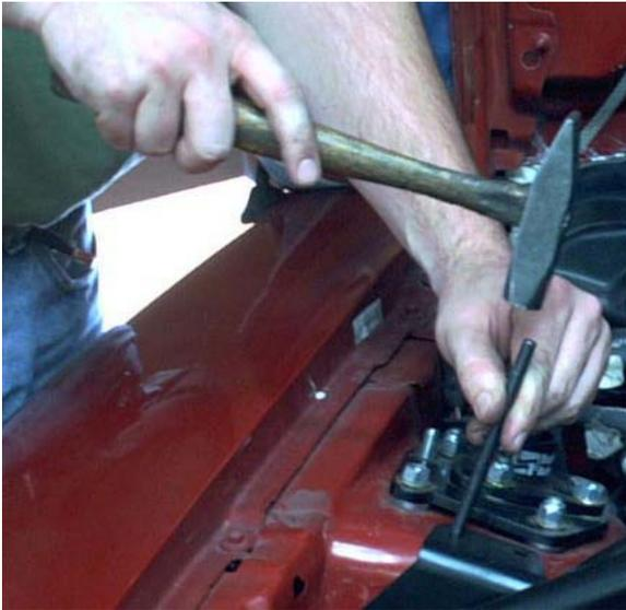
13. Center punch the mark. Drill a 1/8" pilot hole. Drill out to 5/16". Deburr the hole.
