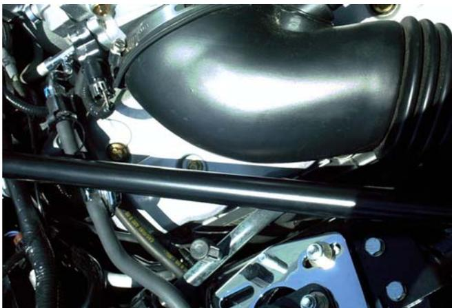
6. Be sure that both firewall mounts of the brace are held down against the firewall pinchweld. Mark the position of the firewall mounts on the plastic firewall cover. The cover will be trimmed in Step 9.
