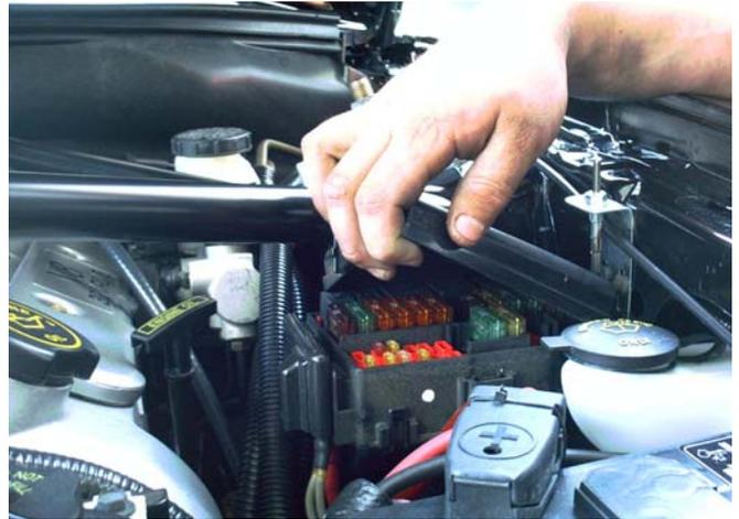
*NOTE: If the fuse box cover cannot be opened, reposition the fuse box by moving it forward. This can easily be done by slipping a screwdriver between the front of the strut tower and the rear of the metal fuse box mounting tabs (these are attached to the strut tower). Gently pry the tabs forward. This will move the fuse box slightly forward.*
