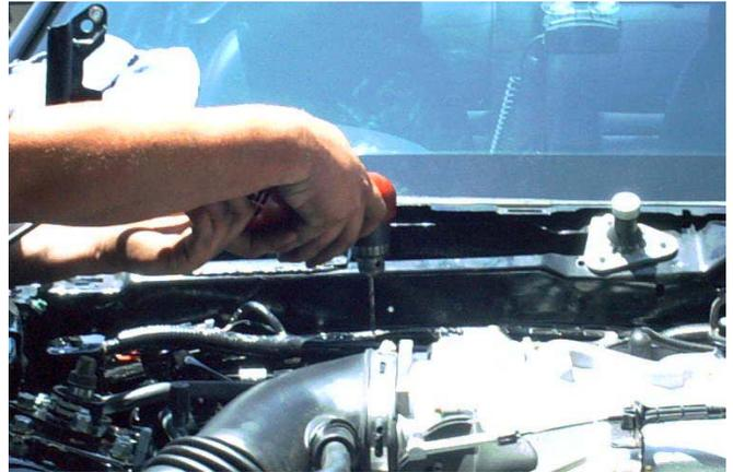
24. Install the 5/16"-18 x 3/4" long bolts in the nutplate. Thread them through so that they protrude on the flat side of the nutplate. It is not necessary to thread the bolts all the way in.
