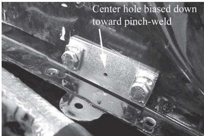
26. Using the nutplate as a template, mark the location of the small hole using a scribe or punch.
