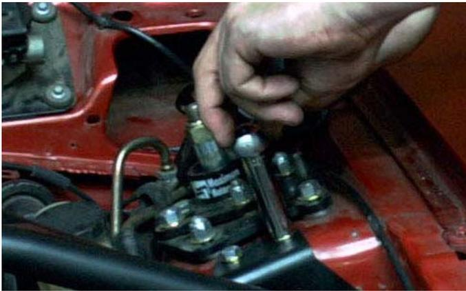
39. Reconnect the hose for the windshield washer nozzles. Reinstall the plastic cowl cover at the base of the windshield by gently snapping it back into position on its clips. Make sure the outer edge of the plastic cowl cover slips past the 'A' pillar applique and into its correct position. Reinstall the 'A' pillar applique bolts previously removed in Step 17.
