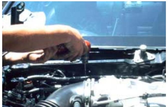
24. Install the 5/16-18 bolts in the nutplate. Thread them through so that they protrude on the flat side of the nutplate. It is not necessary to thread the bolts all the way in.
