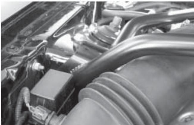
6. Be sure that both firewall mounts of the brace are held down against the firewall pinchweld. Mark the position of the firewall mounts on the plastic firewall cover. The cover will be trimmed in Step 9.
