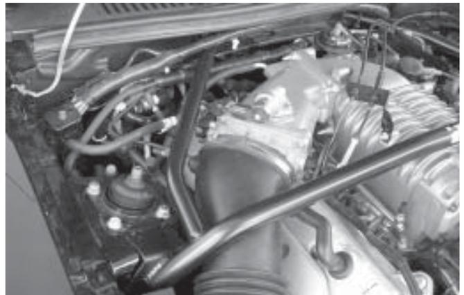
Note: The firewall mounting pads must be routed underneath the wiring harness and the cruise control cable as shown in the photos below.
