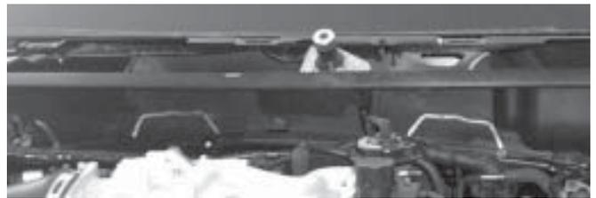
8. Remove the alarm siren (if so equipped) from the firewall. Remove the hood seal from the cowl. Then remove the plastic firewall cover. It is held on with several small sheet metal screws.
