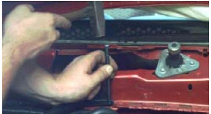
22. Remove the 6 bolts at the strut towers. Remove the Strut Tower Brace.
