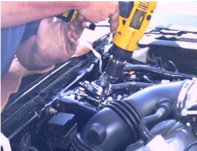
14. Set the Strut Tower Brace back into place. Insert a 5/16" x 1" long bolt into the hole to hold the brace in position. Hold it both downwards and rearwards. Mark the positions of all of the other holes on both strut towers. Unclip the relay box from the inner fender panel to provide access for marking and drilling the hole. Remove the Strut Tower Brace before drilling.
