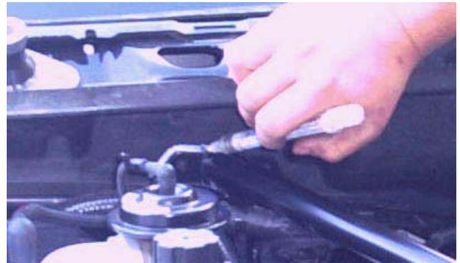
7. Remove the Strut Tower Brace.
