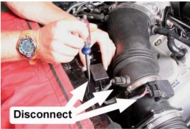
7. Unbolt the pressure sensor located on the driver side of the supercharger and remove the two vacuum lines and electrical connector that are attached to it. The pressure sensor needs to be bolted on the opposite side of the mounting bracket to provide clearance for the strut tower brace.
