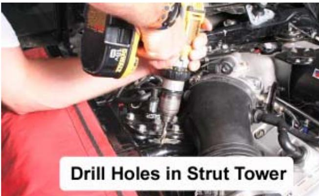
22. Set the Strut Tower Brace back into place. Insert a 5/16" x 1" long bolt into the hole to hold the brace in position. Hold it both downwards and rearwards. Mark the positions of all of the other holes on both strut towers. Unclip the relay box from the driver side inner fender panel to provide access for marking and drilling the hole. Remove the Strut Tower Brace before drilling.
