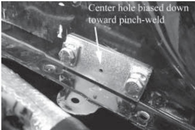
33. Using the nut plate as a template, mark the location of the small hole using a scribe or punch.
