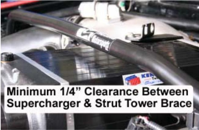
14. Be sure that both firewall mounts of the brace are held down against the firewall pinch weld. Mark the position of the firewall mounts on the plastic firewall cover. The cover will be trimmed in Step 17.
