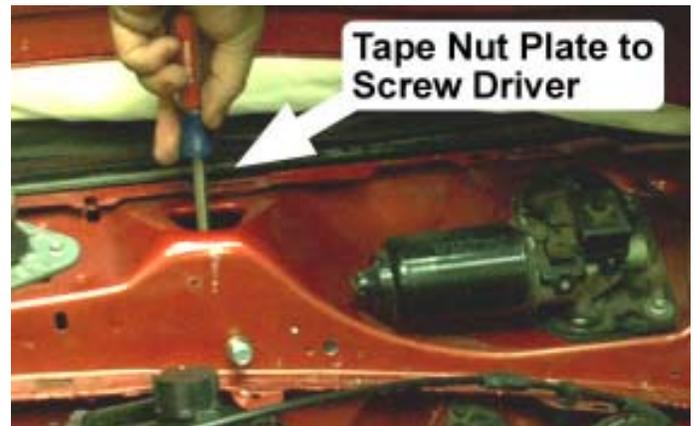
40. Install the #8 sheet metal screw into the small hole in the nut plates. Remove the 5/16-18 bolts.
