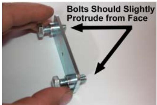
32. Line up the nut plate on the 5/16" holes drilled in the firewall in Step 30. Use the bolts installed in the previous step as guide pins. Make sure that the small hole in the plate is biased downward.
