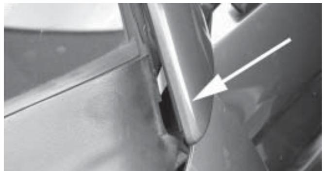
26. Remove the plastic cowl cover at the base of the windshield. It is held on with clips. Remove it by gently prying it upwards. When it is loose, disconnect the hose to the windshield washer nozzles (pointed to, below).
