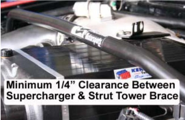
14. Be sure that both firewall mounts of the brace are held down against the firewall pinch weld. Mark the position of the firewall mounts on the plastic firewall cover. The cover will be trimmed in Step 17.
