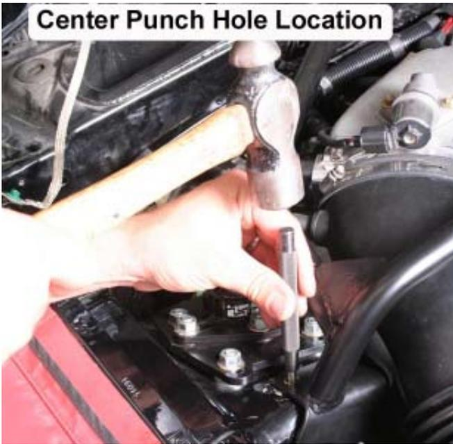
21. Drill a 1/8" pilot hole. Drill out to 5/16". Deburr the hole.
