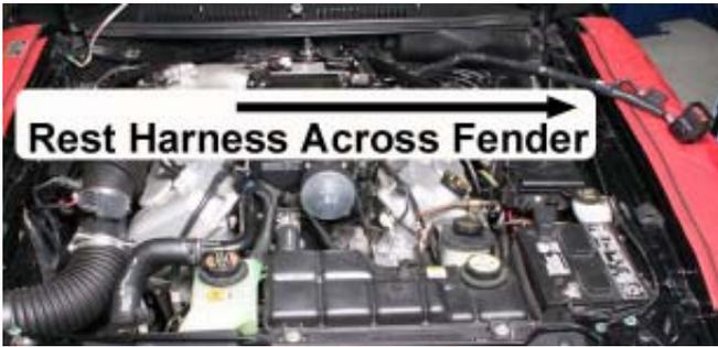
5. Unclip the wiring harness and the cruise control cable from the pinch weld seam at the firewall.
