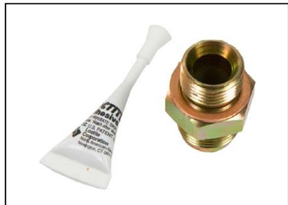
29b. If installing kit OC-2 (w/o thermostat), coat the tapered pipe threads of two AN to pipe fittings with Loctite Thread Sealant. **DO NOT COAT FIRST THREAD.**
