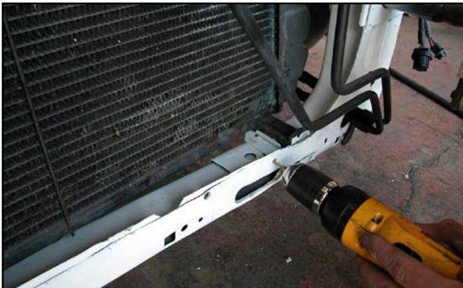
14. Place a 5/16 AN washer under the head of a 5/16" X 3/4" bolt. Position the bolt through the hole drilled in the L-bracket and radiator core support. Place a 5/16 AN washer on the backside of the radiator core support followed by a 5/16 nylock nut. Snug but do not tighten the nylock.
