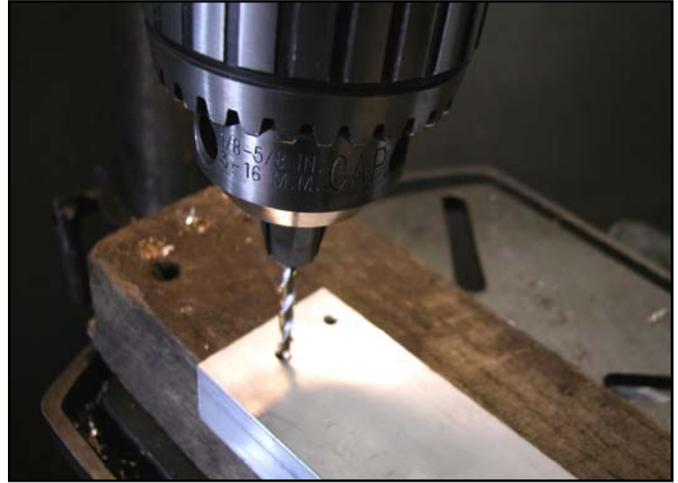
10. On the short leg of the L-bracket, mark a point 1.25" from each end and centered on the leg. Center punch your marks, drill with a 11/32" drill bit and de-burr.
