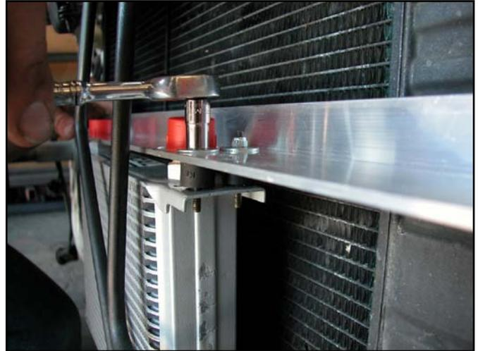
24. Push down on the upper L-bracket and oil cooler assembly to make sure it is fully seated on the lower vibration isolators. Vise Grip the upper L-bracket through the headlight opening.
