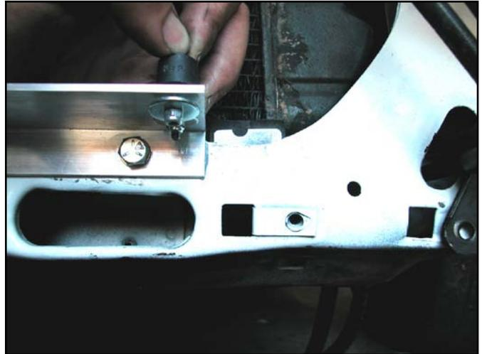
17. With oil cooler placed on vibration isolators, hold upper L-bracket against oil cooler outlets and mark the center of the fittings on the upper L-bracket. Make sure upper L-bracket is centered left-to-right on the car.
