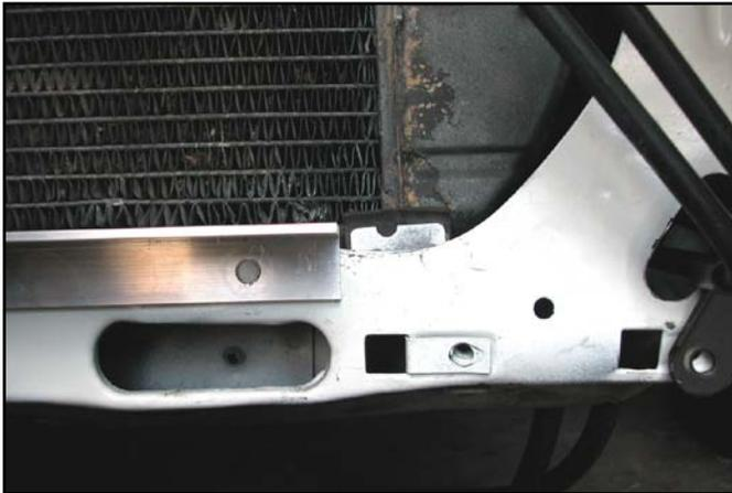
13. Using center punch, mark the center of one of the 5/16" L-bracket holes on lower radiator core support. To ensure accurate placement, **CAREFULLY** drill a pilot hole first, followed by a 11/32" drill bit. If necessary, use a file to de-burr the hole.
