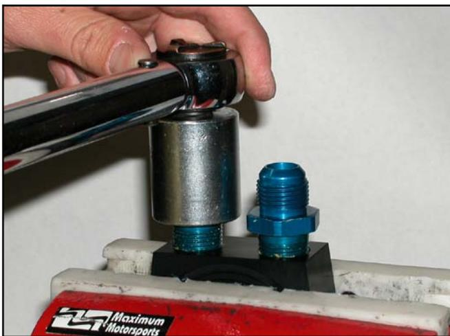
32. Re-install rubber gasket on sandwich block and apply grease to the mating surface. Remove oil filter from the engine and install the sandwich block onto your motor block. **DO NOT** tighten the sandwich block; you will need to be able to rotate it.
