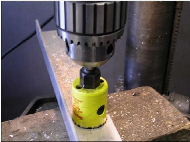
19. Place the upper L-bracket onto the oil cooler and make sure your mark for the second hole still lines up with the second fitting. Repeat step 18 for the second hole. De-burr both of the holes.
