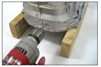
67. Carefully enlarge the hole, using larger and larger drill bits, until the final size is drilled with a 9/16" drill bit.
