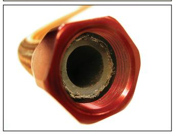
162. Use a felt pen to mark the hose at the base of the socket, so that you can tell if the hose is getting pushed out during the rest of the assembly.
