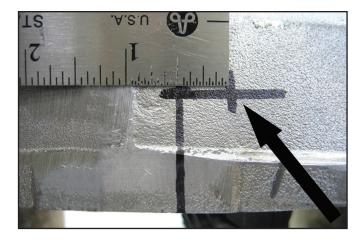
65. Use a center punch to mark the center of the "X".
