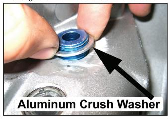
51. Place a few drops of the supplied Blue Loctite® on the threads of bulkhead fitting, adjacent to the aluminum crush washer installed in the previous step.
