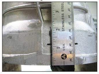
64. Next, measure over ½" to the right of the vertical line, along the horizontal line made in the previous step, and make a small, vertical mark.
