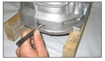
66. Using a 1/8" drill bit, drill a pilot hole through the center punched mark.
