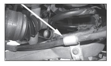
5. Remove the parking brake cable housing retaining clip on each caliper.
