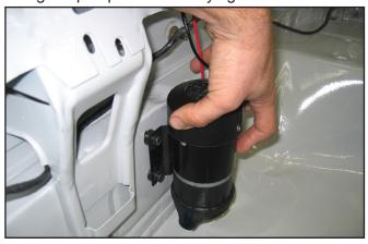
109. Remove the two screws retaining the differential oil pump mounting bracket to the differential oil pump.
