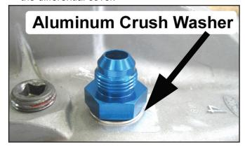
50. Place the remaining aluminum crush washer on the portion of the bulkhead fitting protruding through the inner face of the differential cover.
