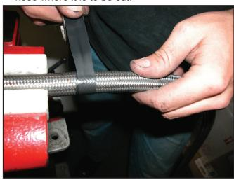
156. Squarely cut through the tape-wrapped sections of the hose using a sharp 32 TPI (or finer) hacksaw blade.
