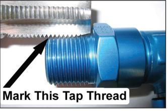
57. Count three full threads on the 3/8" NPT pipe tap, above the mark previously made, and wrap a piece of masking tape around the tap. The masking tape should be wrapped above the third thread. The 3/8" NPT tap is now ready for use.
