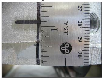
84. Next, measure over 3/8" to the left of the vertical line along the horizontal line made in the previous step and make a small, vertical mark. This would be towards the passenger side of the car, when the case is in the vehicle.
