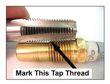
77. Count three full threads on the 1/4" NPT pipe tap, above the mark previously made, and wrap a piece of masking tape around the tap. The masking tape should be wrapped above the third thread. The 1/4" NPT tap is now ready for use.
