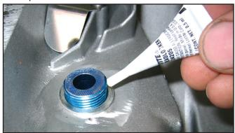
52. Thread the supplied –8AN blue aluminum nut onto the bulkhead fitting.
