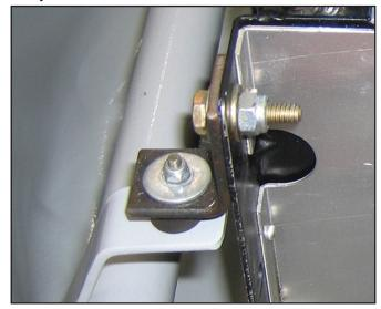
107. Carefully tighten the M4 nylock nuts until they are snug.
