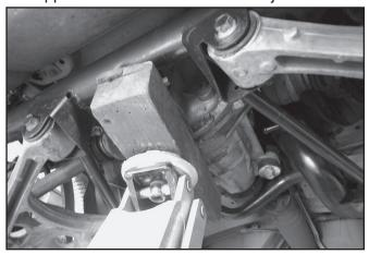
26. Remove the two mounting bolts, located on the differential cover, that attach the cover to the rearward differential bushing.
