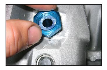
53. Tighten the nut as much as possible by hand, and then use a wrench to tighten the nut a further 3/8 of a turn.
