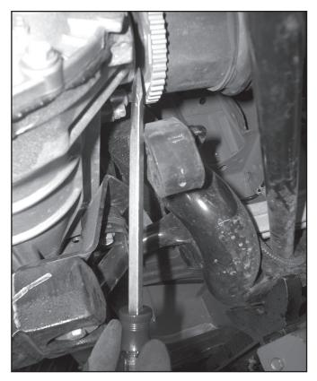
15. Use a floor jack to support the passenger side lower control arm, and remove the lower shockmounting bolt.
