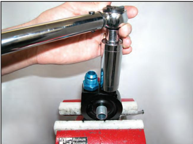
13. Attach the Adapter Plate to the Remote Filter Mount using the three supplied 5/16" bolts. Tighten the three bolts to 19 ft-lb.
