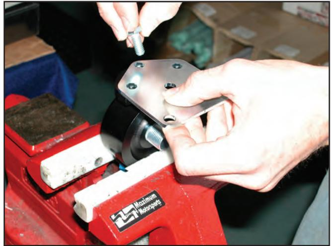
14. Insert one of the self-tapping screws through the center hole in the Adapter Plate from the filter side of the Adapter Plate.
