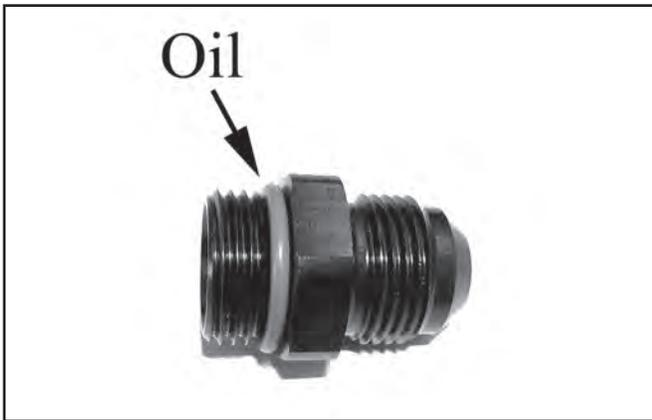
12. Place the Remote Filter Mount into a vise with "soft jaws" and install each of the two Straight Thread O-ring to -10AN fittings into the two ports of the filter adapter. Tighten the adapter nipples to 35 ft-lbs.
