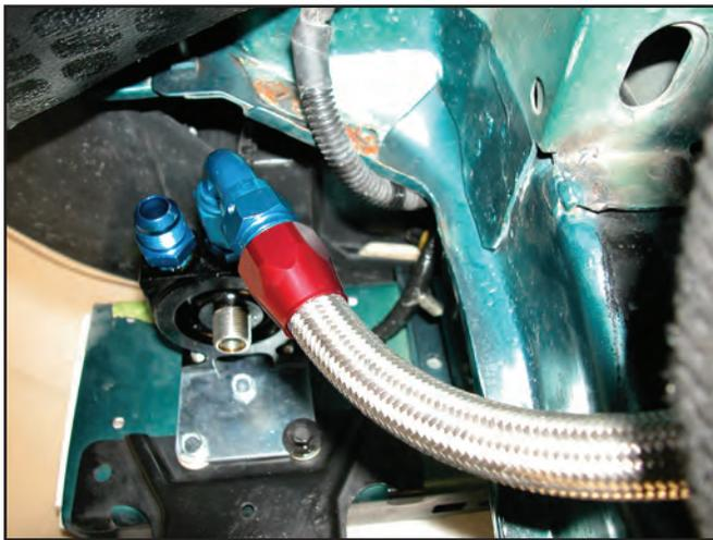
30. Route the hose under the frame rail, over the anti-sway bar and to the Engine Block Adapter. The specific routing should be based on your personal preference and vehicle configuration.
