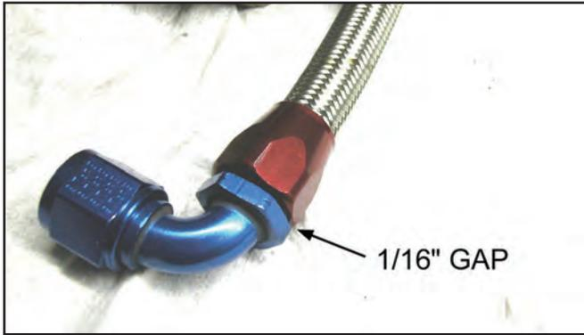
28. Make sure the mark made at the base of the socket at step 25 has not moved relative to the socket by more than 1/16". If it has, remove the fitting and return to step 24.
