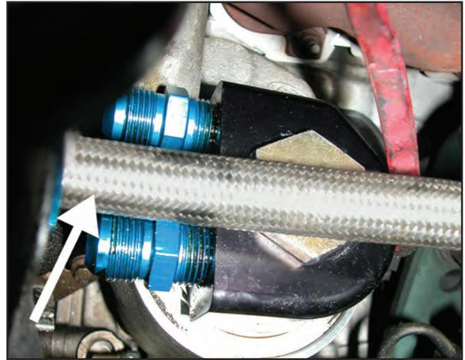
32. Remove the hose from the Remote Filter Mount and remove the hose from the car.
