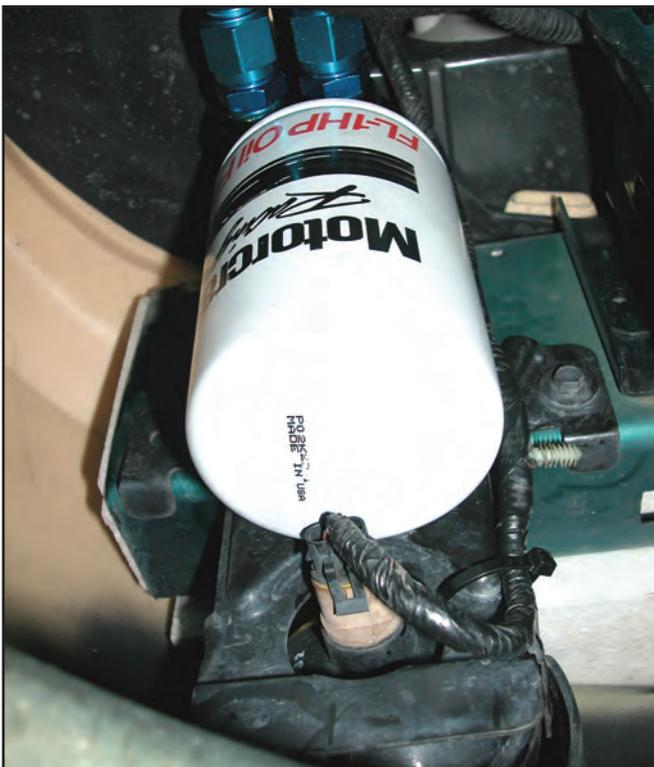
49. Start the engine and examine all of the oil lines and oil line connections carefully to ensure that everything is tight and that there are no leaks. Turn off the engine after examining the oil lines and oil line connections.
