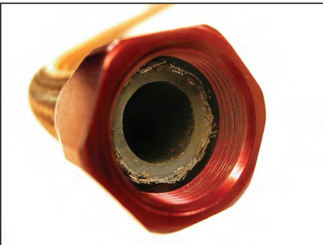
25. Use a felt-tip pen to mark the hose at the base of the socket, so that you can tell if the hose is getting pushed out during the remaining steps of the fitting installation.
