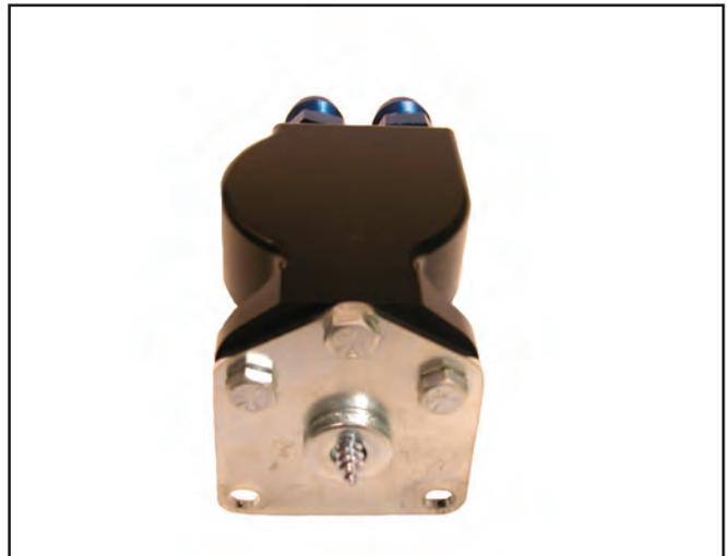
16. Attach the Adapter Plate to the bumper support by inserting the self-tapping bolt into the hole drilled at step 9. Leave the self-tapping bolt loose.
