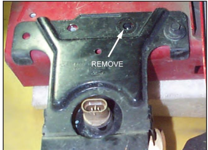
6. Temporarily attach the Adapter Plate to the bumper support using the bolt removed at step 5 in its original position. Thread one of the provided self-tapping bolts at the unused hole in the bumper cover support behind the driving light bracket. The Adapter Plate is now used as a template for locating the position of a third mounting hole for the Adapter Plate.
