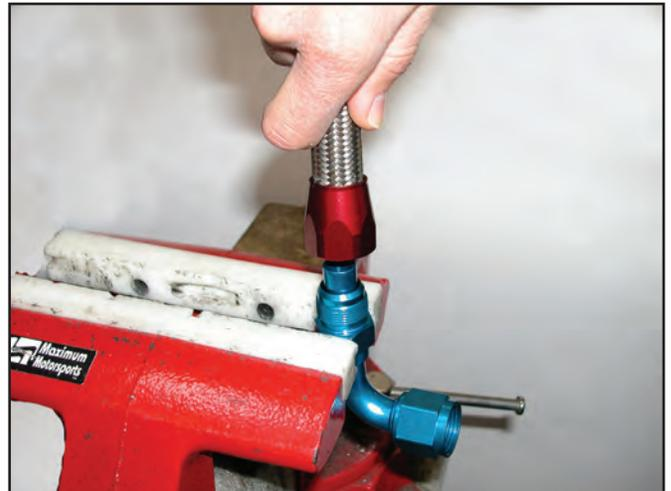
27. When you can no longer tighten the fitting by hand, use appropriate size wrenches to tighten the fitting. Tighten the fitting until the red socket is within 1/16" from bottoming on the blue nipple. Do NOT use adjustable or oversize wrenches, or you will damage the fitting.
