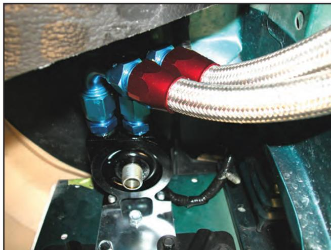
42. Attach the STRAIGHT fitting of the SECOND oil line to the upper adapter nipple of the Engine Block Adapter and tighten to 15 ft-lb.
