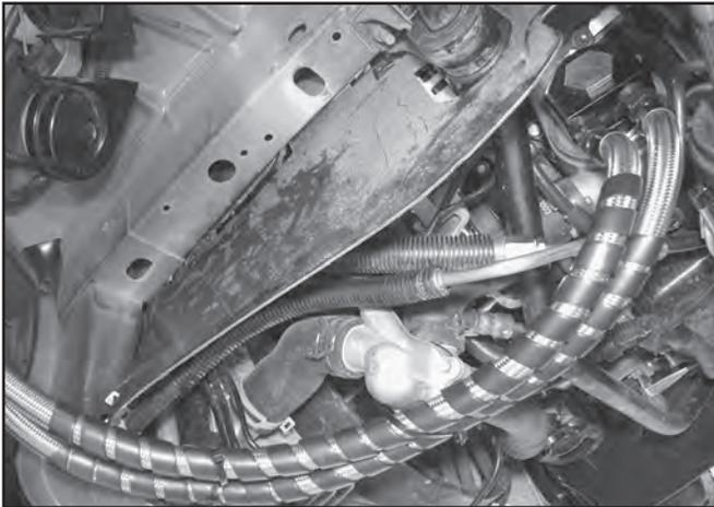
46. Use the supplied zip ties to secure the oil lines as needed.
