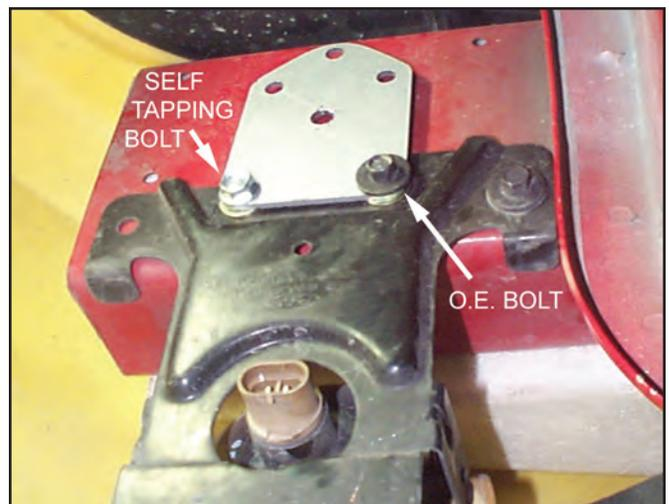
7. Mark the location of the center hole of the Adapter Plate on the bumper support.
