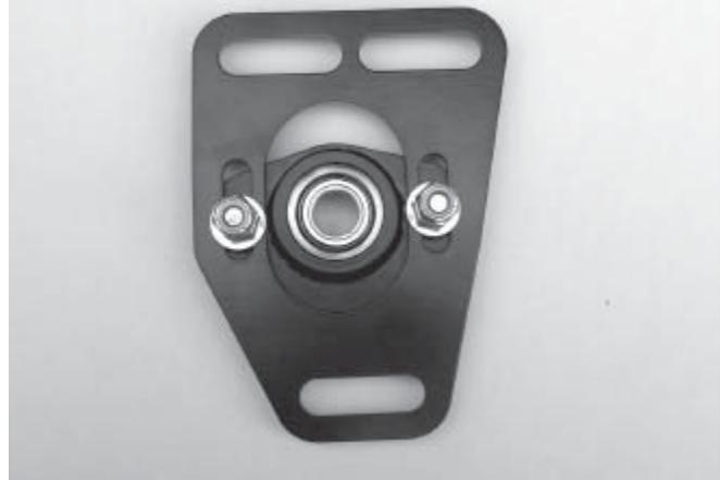
19. On each side of the car, install the appropriate Main Plate with the Bearing Plate mounted to its underside.
