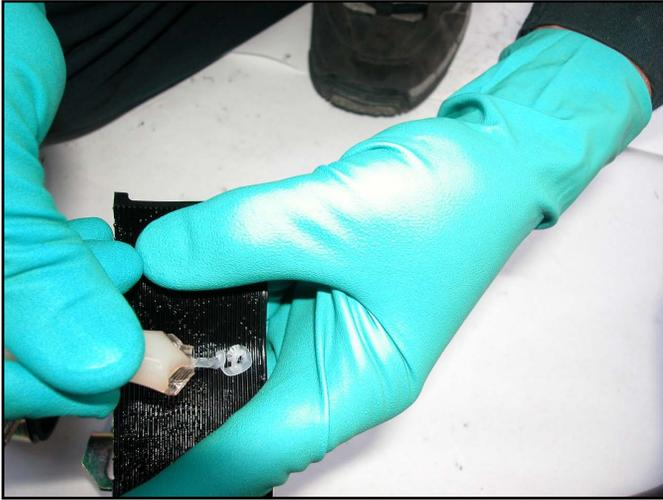
11. Place the greased urethane bushing onto the swaybar.
