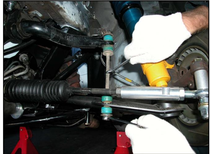
6. Remove stock U-bracket from the swaybar. TIP: Use a large screwdriver to pry off retaining plate.
