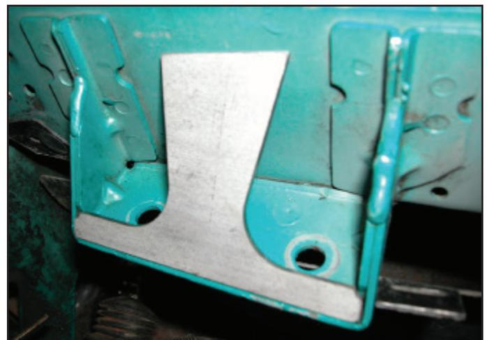
8. Mark with a Sharpie pen or grease pencil all areas where the MM Reinforcement contacts the frame rail.
