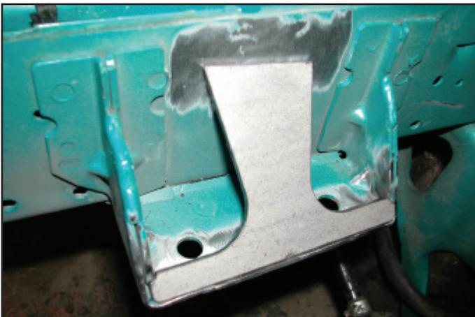
11. Weld all areas where the MM Reinforcement contacts the OEM sheet metal. Use a MIG or TIG welder. If using a MIG welder, be sure to protect the engine with a welding blanket. If you are unsure of your welding skills, have a professional welder perform this operation. It is recommended to prime the backside of the MM Reinforcement, preferably with weldable primer.
