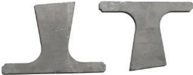
The 1979-93 Mustang front swaybar mount is spot welded into place. Because it hangs off the frame rails, it is prone to flexing and commonly develops cracks. The MM Front Swaybar Bracket Reinforcement braces the factory swaybar mount to prevent flexing and stop cracks from developing.
