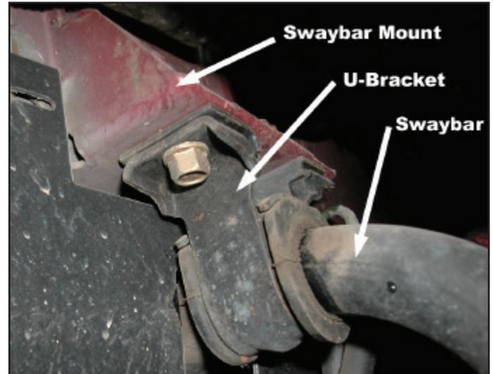
6. Inspect the swaybar mount for existing cracks and weld the cracks as necessary.
