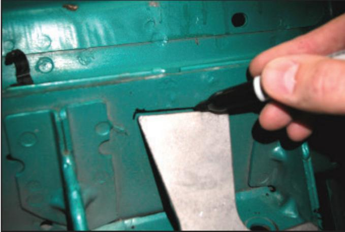
9. Remove the MM Reinforcement. Wire wheel or sand, to bare metal, all areas to be welded.
