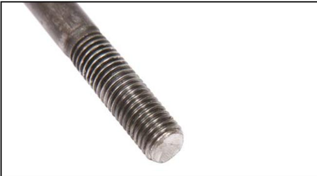
90. Reinstall the trimmed steering rack bolts, from the front of the k-member.
