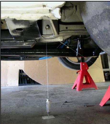
48. Wait for the plumb bob to stop swinging. Mark the position of each plumb bob by placing a small dot on the tape directly under the tip of the plumb bob.
