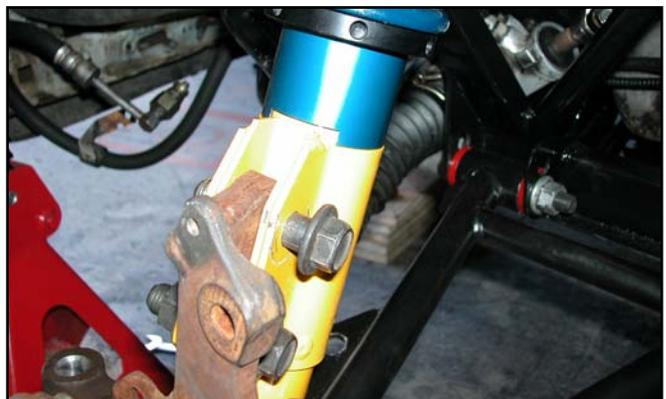
104. Attach the adjustable outer tie-rod end to the spindle. As a starting point, place a 2" stack-up of spacers between the spindle and the tie-rod end. Torque the tie rod end bolt through the spindle to the specification of your bump steer correction kit.
