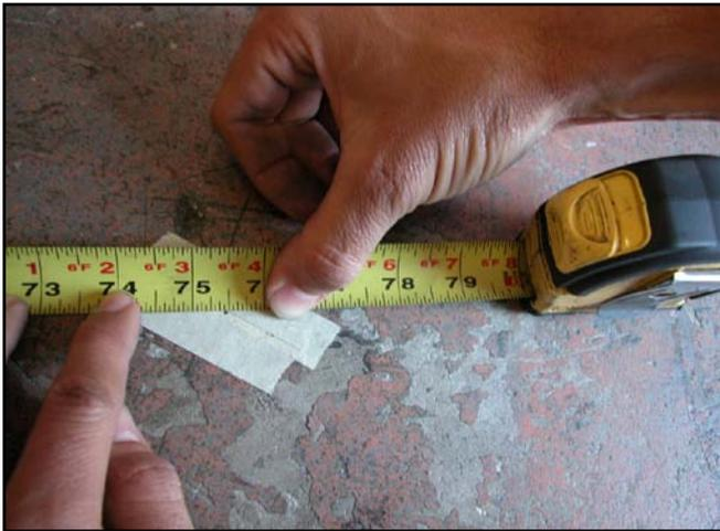
55. Take the same measurement between the two dots on the right side of the car.
