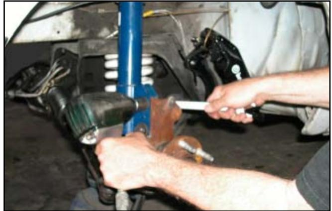
14. Loosen the tie-rod end nut but do not remove it.
