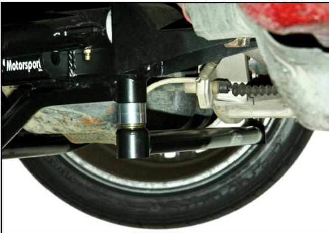
41. Place a board on the floorjack and place the K-member on the board. The K-member should be located so that it is balanced on the center of the jack pad.
