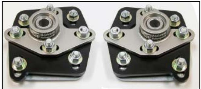
101. Install a front coil-over conversion kit now if the car is not yet so equipped.
