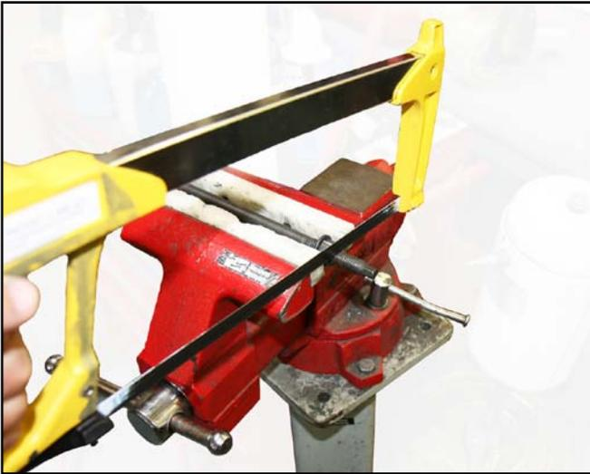
89. You will need to chamfer the edges of the cut bolts and clean the threads with a file so the OEM Ford nuts will easily start to thread onto the bolts. The bolt thread is M12 x 1.75. If you have a thread file or a die set, this can be used to clean up the threads after a chamfer has been put on the end with a file. After the bolt tips are dressed, remove the nuts as the final Step to ensure the threads are properly formed.
