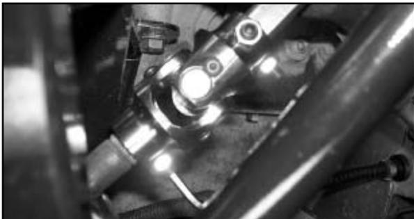
97. If using the forward-offset MM control arms, now is the time to move the swaybar forward 1" with the appropriate MM Relocation Kit (MMFSB-50,-51).
