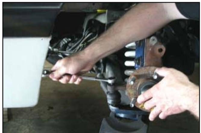
15. Spray the outer tie-rod end taper stud with penetrating oil.
