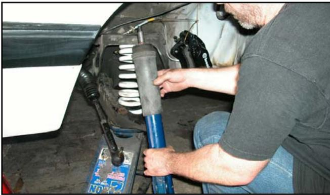
28. Carefully lower the floor jack until the front spring becomes unseated from the upper spring perch.
