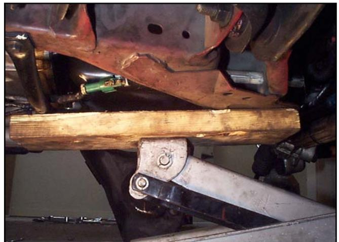
36. Loosen, but do not remove the four bolts that hold the K-member to the frame near the upper spring perches.
