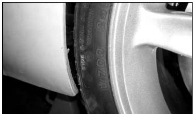
AFTER TRIMMING THE FENDER EXTENSION
