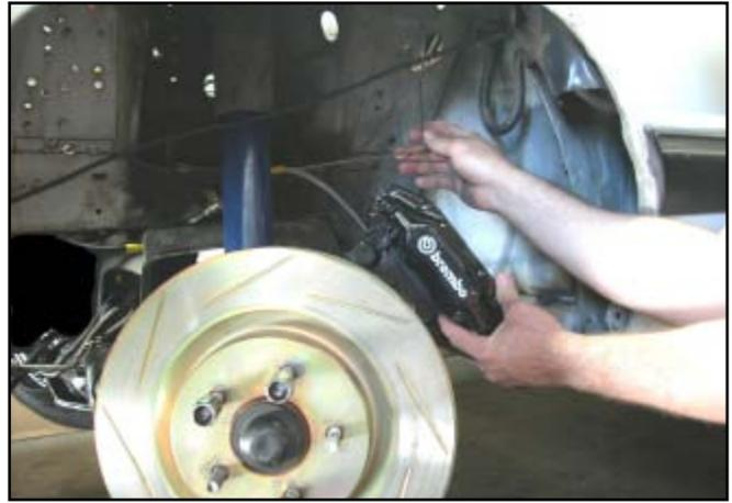
11. Remove the front brake rotor.
