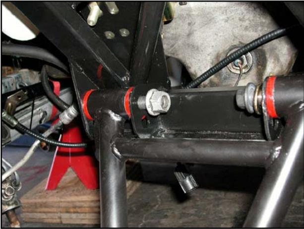
82. Hold the head of the MM Low Profile Front Control Arm Bolt stationary using a T-55 Torx socket and tighten the nut. Torque the nut to 148 ft-lbs.
