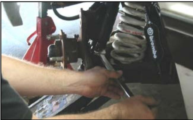
19. Spray the ball joint taper with penetrating oil.
