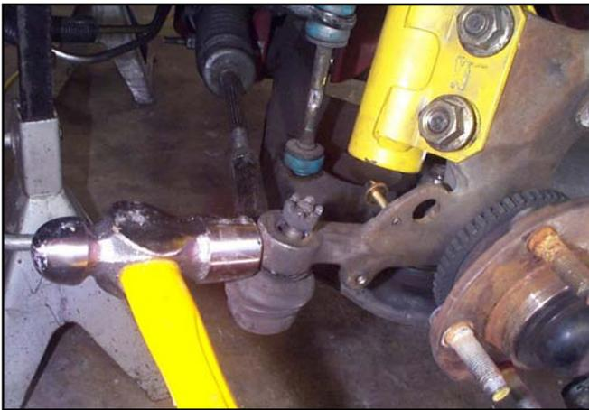
20. Remove the nut from the tie-rod end and detach the tie-rod end from the steering arm.
