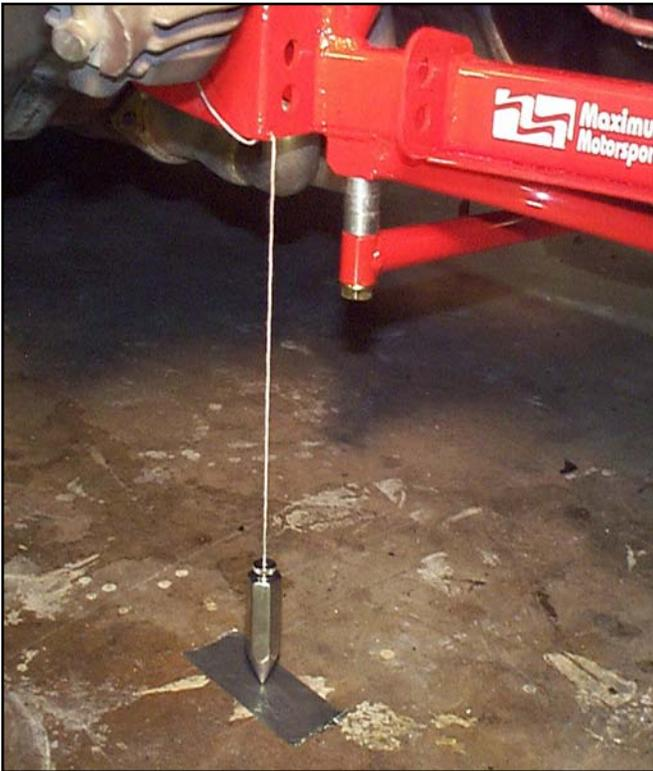
52. Wait for the plumb bob to stop swinging. Mark the position of each plumb bob by placing a small dot on the tape directly under the tip of the plumb bob.
