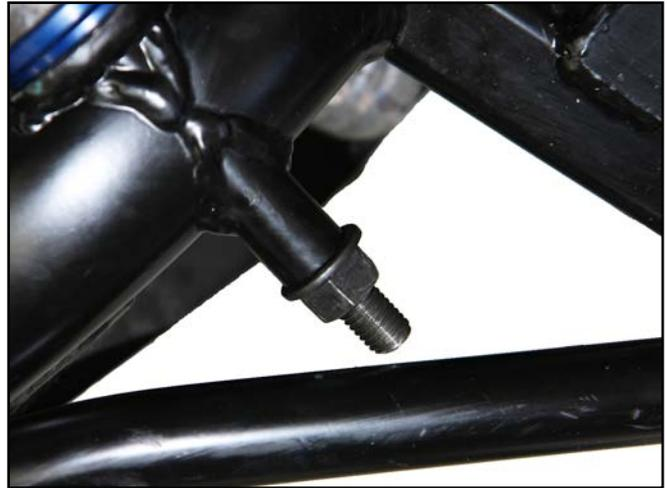
91. Snug the factory nuts onto the steering rack bolts. With offset steering rack bushings, ensure that the bushings as well as the spacers behind the rack are oriented correctly. The three holes in each bushing should be in a vertical line with the center of the bushing.
