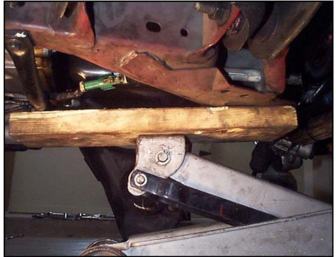
35. Loosen, but do not remove, the four bolts that hold the K-member to the frame near the upper spring pockets.
