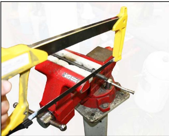
88. You will need to chamfer the edges of the cut bolts and clean the threads with a file so the OEM Ford nuts will easily start to thread onto the bolts. The bolt thread is M12 x 1.75. If you have a thread file or a die set, this can be used to clean up the threads after a chamfer has been put on the end with a file. After the bolt tips are dressed, remove the nuts as the final step to ensure the threads are properly formed.
