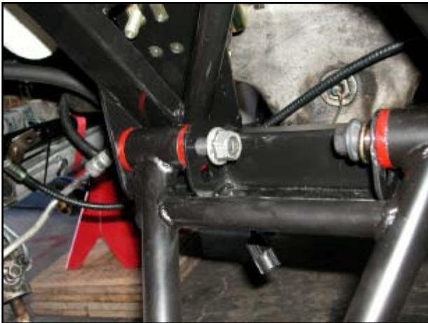
81. Hold the head of the MM Low Profile Front Control Arm Bolt stationary using a T-55 Torx socket and tighten the nut. Torque the nut to 148 ft-lbs.
