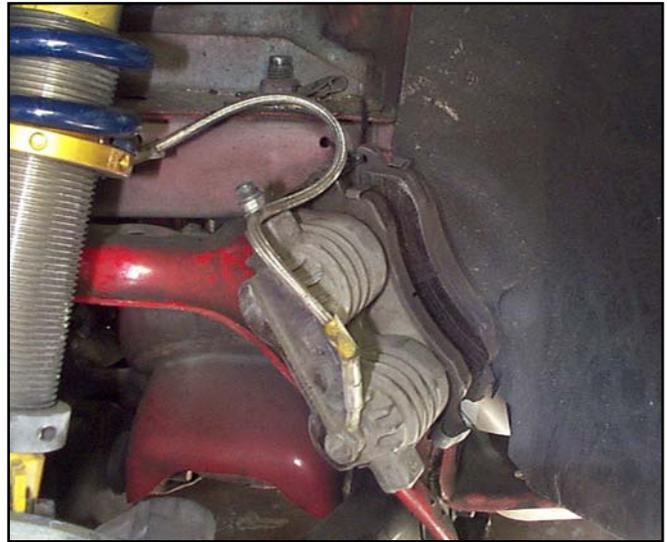
10. Remove the front brake rotor.
