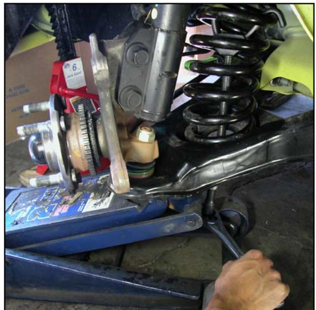
23. Raise the control arm 1/2" with the floor jack. Remove the ball joint nut completely.
