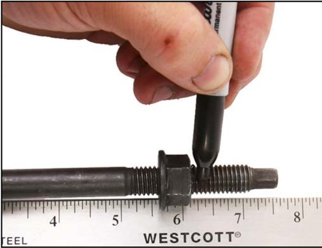
87. Use a hack saw or grinder to cut each bolt at the mark placed in Step 86.
