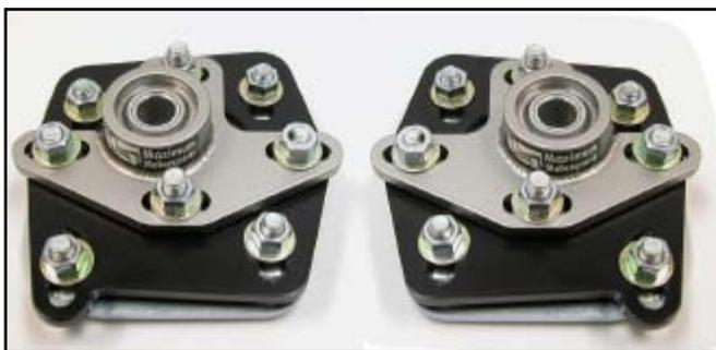
99. Install a front coil-over conversion kit now, if the car is not yet so equipped.
