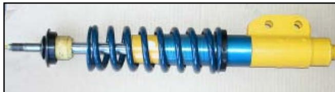
100. Install the coil-over strut assembly into place in the caster/camber plate. Adjust the spacers between the upper spring perch and the caster/camber plate as per the MM Front Coil-over Kit instructions to allow for maximum bump travel.
