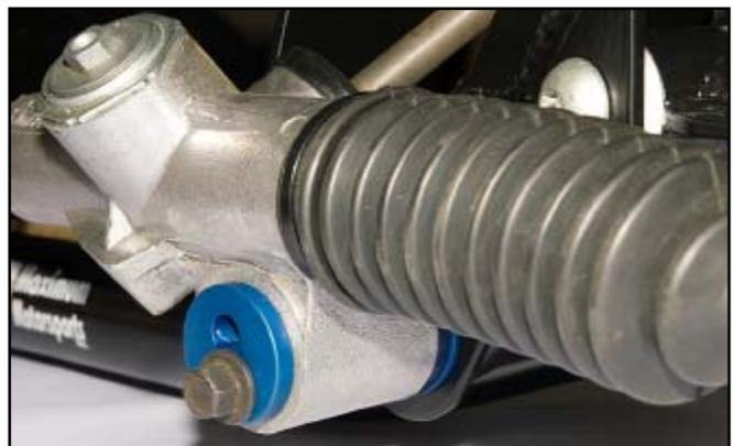
92. Torque the steering rack mounting bolts to 55 ft-lbs.
