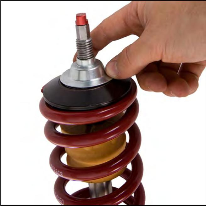
20. Place the passenger side MM Caster/Camber Plate assembly onto the strut shaft by slipping the shaft through the spherical bearing.
