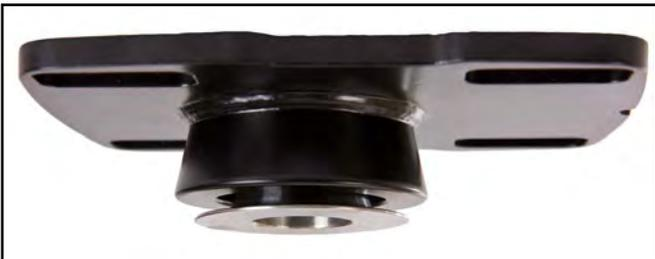
21. Place the spacer stack configuration shown below onto the strut shaft. Ensure that the tapered spacer is properly seated in the spherical bearing.
