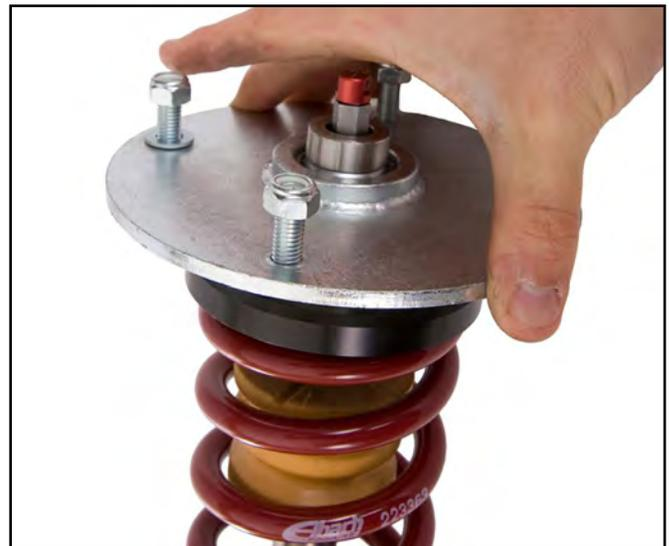
13. Remove the upper spring perch from the Eibach strut assembly.
