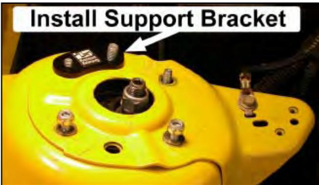
25. Place one of the provided large G8 washers on to the Caster Plate Stud, followed by one of the provided 10mm Nylock nuts and thread it on until the tip of the bolt touches the Nylock portion of the nut.
