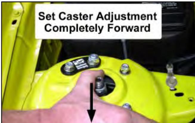
31. Next, center the strut shaft in the strut tower opening side to side. Once centered, torque the four 8mm Nylock nuts to 20 lb-ft.
