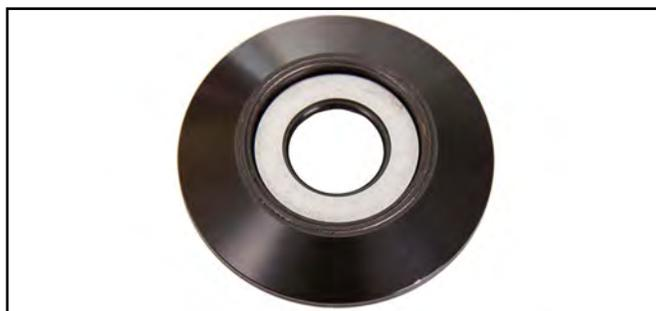
16. Pack the Thrust Bearing with a high quality Moly wheel bearing grease and place it on top of the installed Thrust Washer.
