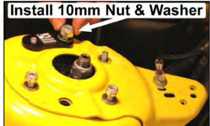
26. Place one of the provided small G8 washers onto each of the remaining studs, followed by the provided 8mm Nylock nuts, and thread them on until the tip of the bolt touches the Nylock portion of the nut.
