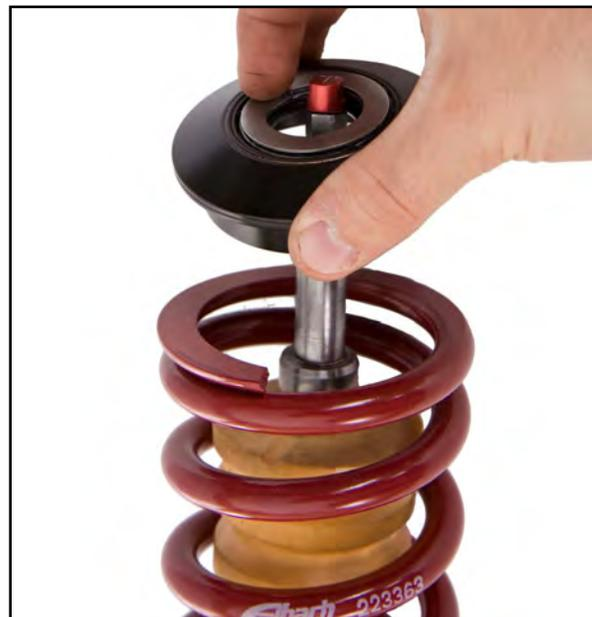
*NOTE: Make sure the Upper Spring Perch is below the shoulder on the strut shaft when tightening the assembly in Step 22. If the perch is shifted to one side, it could bind and prevent the locknut from securing the assembly.*
