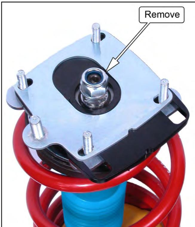
11. Discard the old Spring Perch (shown below), and any of the existing spacers. Pliers may be needed to remove any spacers inserted into the spherical bearing.
