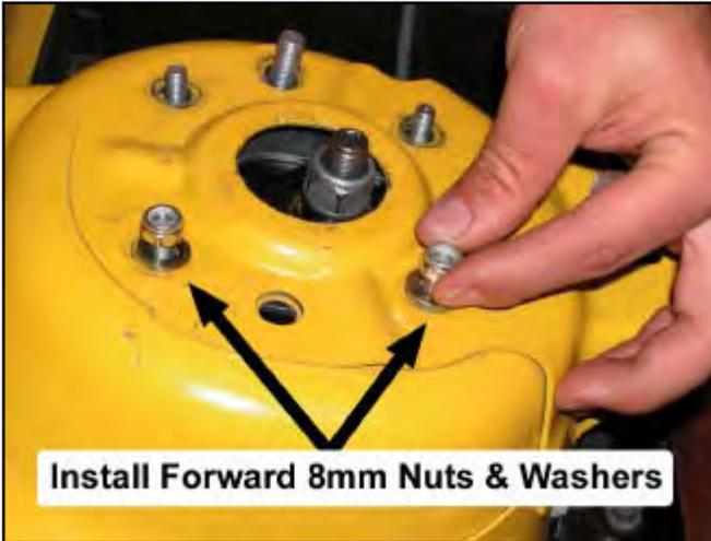
24. Place the passenger side Support Bracket onto the protruding studs, as shown in the photo. The Support Bracket should be oriented towards the outboard side of the vehicle.
