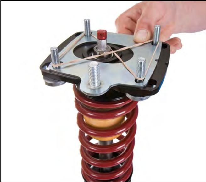
*NOTE: Make sure that the Thrust Cone is fully seated inside of the Bearing as shown below. If this is not installed correctly, the assembly will make noise.*
