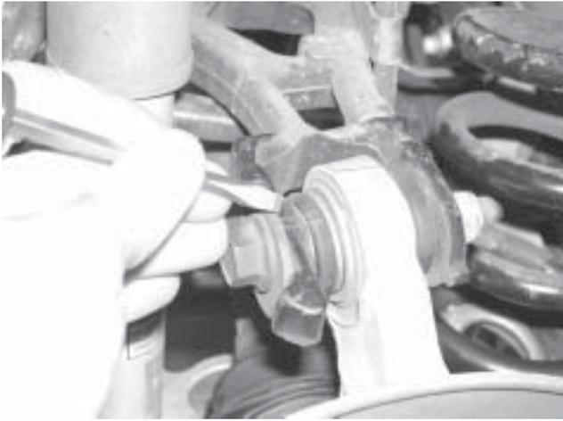
19. Loosen the upper spindle mounting bolt on the passenger side control arm.
