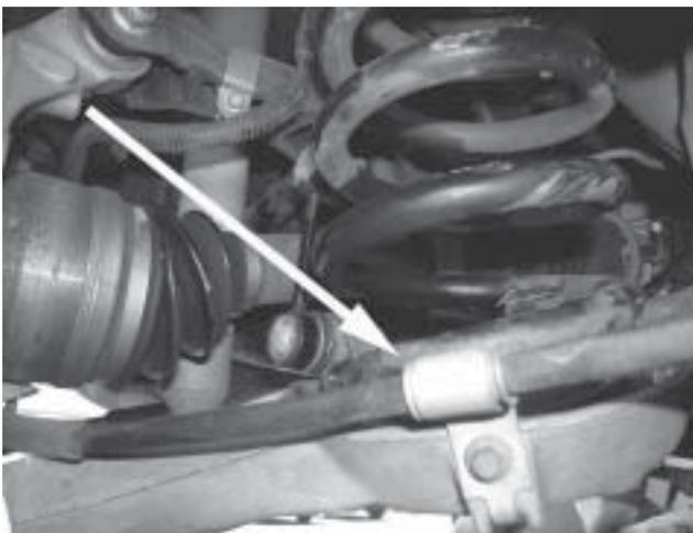
17. On 2003-04 vehicles, remove the brake line locator brackets from the control arms. It will be necessary to spread the bracket legs apart in order to remove them.
