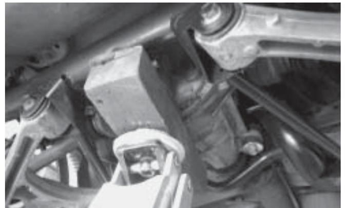
28. Remove the two rear 12mm IRS subframe mounting bolts.
