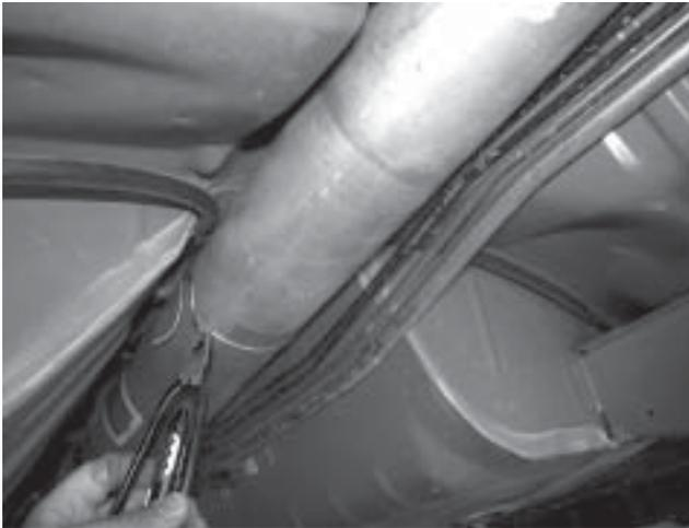
15. Disconnect the parking brake cable from the parking brake lever on each caliper. Remove the cable from the locating hole in the calipers.
