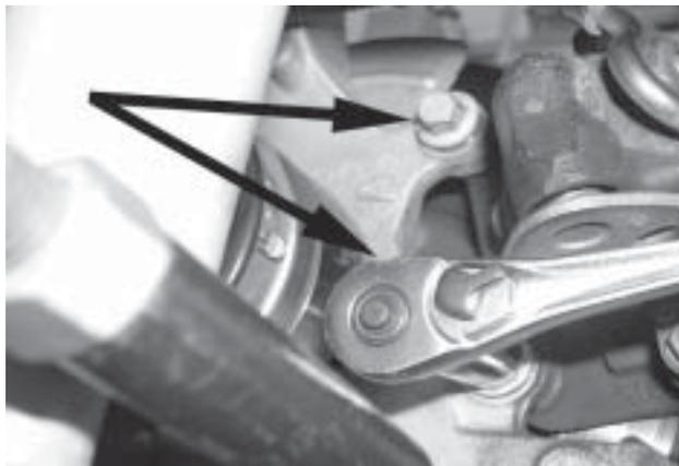
21. Remove the upper spindle mounting bolt.
