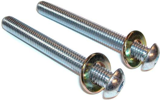
Thank you for buying the Maximum Motorsports Low-profile IRS Rear Sub-frame Bolts. These bolts provide the maximum space possible for inside tire clearance on IRS-equipped cars. The head on our low-profile bolt is 30% shorter than the stock bolt. In addition, the rounded shape will be more gentle on the tire sidewall should a little bit of tire rub occur.
