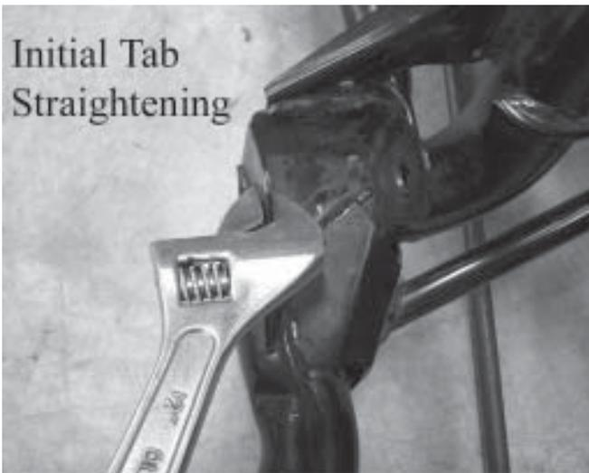
27. Set the cup tool on the outside of the tab. Place the 3/8 flat washer under the bolt head. Run the bolt through and place the thick washer and nut on the inside of the tab. Use anti-seize or oil on the threads and washer surfaces.
