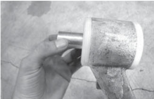
31. Install the arms into the sub-frame. Snug the mounting bolts, but do not fully torque. The arms will be removed again later. Note: You will notice a gap between the bushings and the mounting tabs, especially at the front set of tabs. This is to be expected, and will be taken up with the shims.
