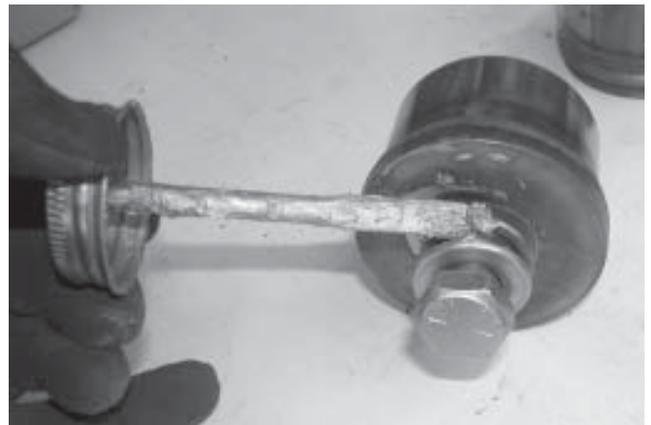
12. Apply anti-seize between the washers, the head of the bolt, and the removal cup.
