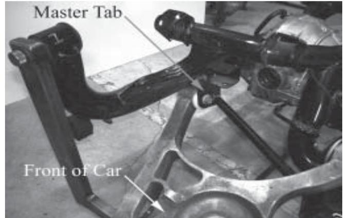
33. On all of the other bushings, open up a gap between the bushing shoulder and the control arm shoulder by pulling the bushings away from the arm, toward the mounting tab surface as shown.
