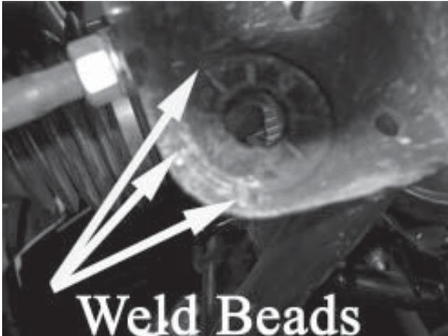
21. Using a small cut-off wheel attached to a drill or die-grinder, grind through the weld beads attaching the spacer to the tab. DO NOT grind deeper than necessary, the surface must be smooth for the MM delrin bushings to function properly.
