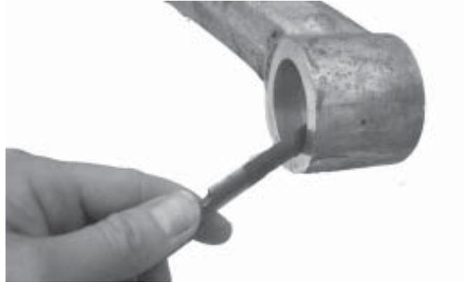
20. Using the supplied Scotch-Brite pad, remove any rust residue from the steel shell and smooth out any rough spots. When finished, wipe the area with a clean rag.
