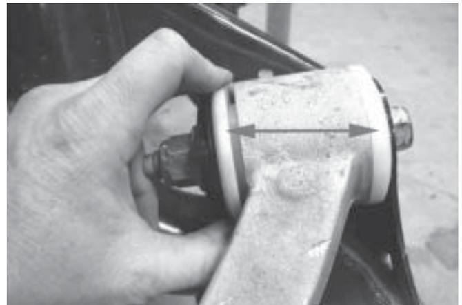
Note: There are four types of shims provided with each kit: Large diameter shims (thick and thin) for the large bushings, and small diameter shims (thick and thin) for the smaller bushings. More are provided for the smaller bushings since they will require thicker shim stacks.
