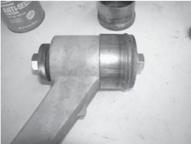
15. Thread the supplied 5/8" nut on to the bolt.
