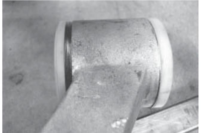
38. Reinstall the arms on the car. Snug, but do not fully torque, the pivot bolts.
