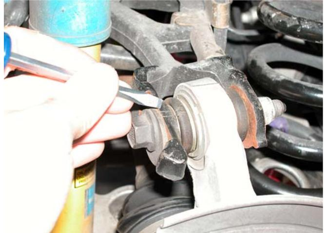
9. Remove the mounting bolts securing the upper and lower control arms to the spindles.
