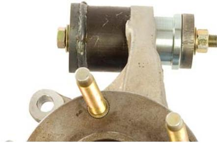
29. Using a pair of wrenches, draw the MM Cross-Axis Joint into the aluminum spindle by tightening the bolt until it runs out of threads. Switch to the shorter bolt when this happens, and finish drawing the Joint into the spindle until the flanged portion is resting against the face of the spindle.
