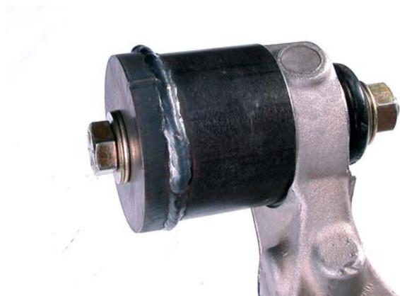
20. Using a pair of wrenches, tighten the bolt to pull the bearing into the Removal Cup.
