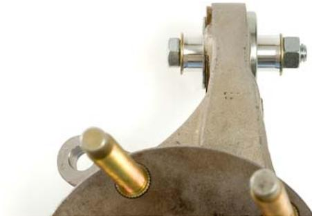
38. Draw the Bearing Insert into the spherical bearing by tightening the bolt with a pair of wrenches. Make sure the Insert seats flush against the face of the spherical bearing.
