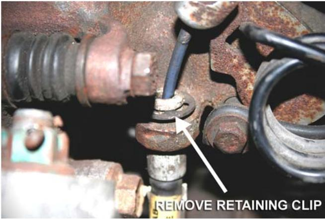
4. Disconnect the parking brake cable from the parking brake lever on the caliper, and remove the cable from the locating hole in the caliper.
