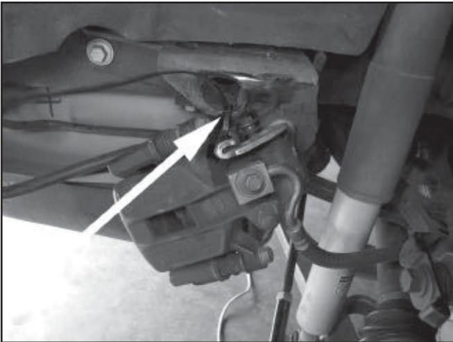
8. Remove the cotter pin and nut that secure each tie-rod end to the rear spindle.
