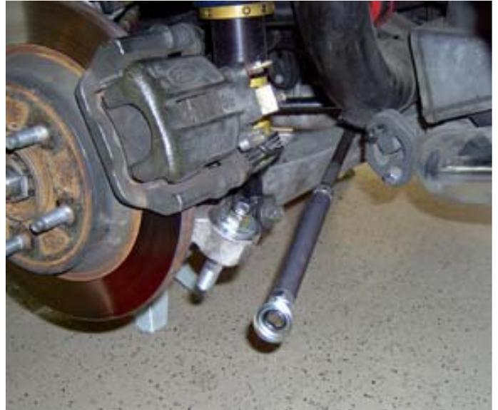
14. Slip the .060" thick spacer onto the bottom of the tapered stud. This spacer will make the bumpsteer curve approximately the same as the 2003 Cobra. In the absence of measuring the bumpsteer on your car, MM recommends this bumpsteer geometry for cars retaining the rubber bushings in the rear suspension.
