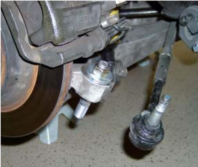
Note: The shoulder of the tapered stud will not contact the bottom surface of the steering arm. The shoulder is designed to provide a stop for the spacers in your MM Kit. The tightly controlled taper dimensions (both on the Ford steering arm, and on the MM Tapered Stud) control how deep the stud sets into the tapered hole.
