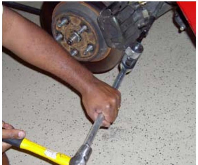
10. Install one of the supplied tapered studs through the steering arm of the spindle. Secure the tapered stud to the steering arm using one of the supplied washers and 1/2-13 lock nuts. Torque the lock nut to 50 ft-lbs.
