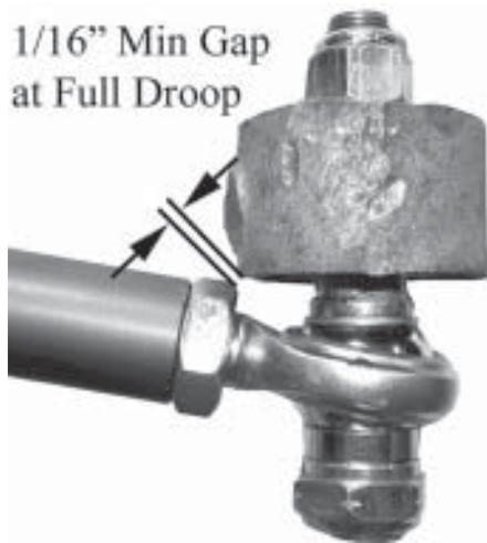
21. The length of the tie-rod assembly is adjusted by rotating the tie-rod. Lengthen the assembly to match the dimension recorded in Step 4.
