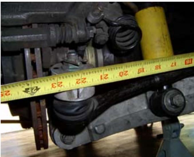
8. Remove the nut securing the tie-rod end to the spindle. Apply penetrating oil to the tie-rod end where it comes through the spindle.
