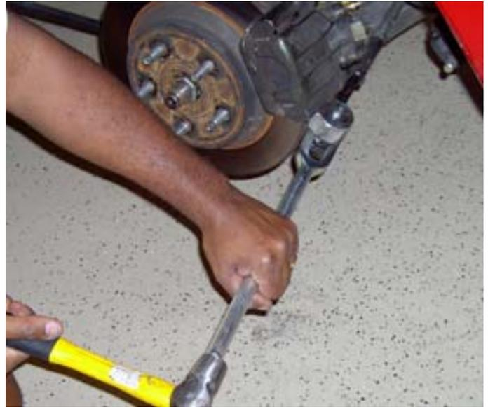
10. Remove the bolt securing the inner tie-rod end to the IRS sub-frame and remove the factory tie-rod from the vehicle.
