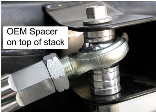
Note: Raising the inner tie-rod pivot by placing additional spacers below the tie-rod end will have the same effect on bumpsteer as lowering the outer tie-rod end.
