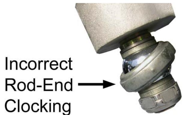
25. Tighten the tie-rod end jam nuts to 41 ft-lbs.
