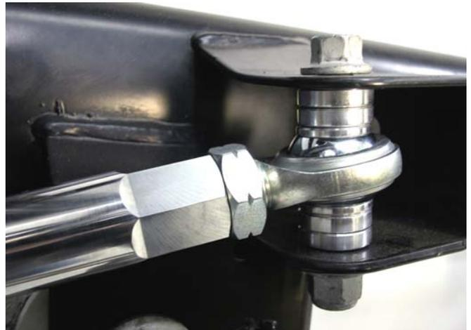
Note: MM recommends a spacer stack that is biased upwards (3 below, 1 above) as a starting inner-spacer configuration for **2003-04 IRS** cars. Place the OEM Spacer on the top of the MM spacer stack (OEM Spacer not shown in photo).
