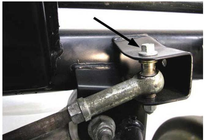
Note: 2003-04 cars have a factory spacer installed between the upper mounting tab and the tie-rod end crush sleeve. Keep this part. It will be re-used.
