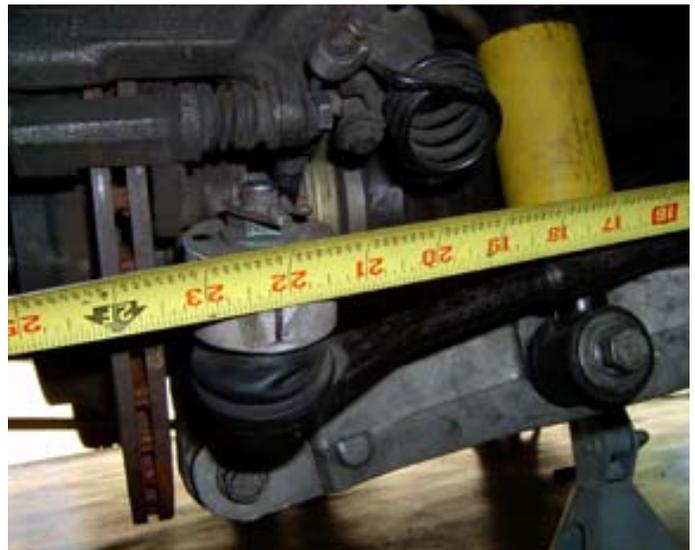
6. Make a record of the spacer configuration where the spherical rod-end attaches to the tapered stud of the MMIRSTR-1 kit. It will be needed later. Remove the 5/8" nylock nut securing the outer tie-rod end to the MM Tie Rod Stud.
