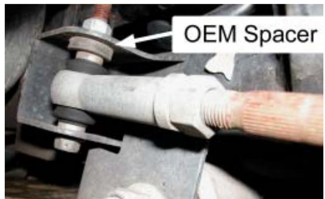
Note: With the tie-rod removed from the vehicle, you may wish to match the length to your new MM tie-rod now. You can do this by loosening the jam nuts on the new MM tie-rod and adjusting the length so that the center to center distance between the tie-rod mounting holes matches the tie-rod removed from the vehicle. Be certain to adjust both ends equally. This can save effort under the car, and a trip to the alignment shop if done properly.
