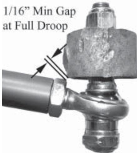
17. The length of the tie-rod assembly is adjusted by rotating the tie-rod. Lengthen or shorten the assembly to match the dimension recorded in Step 5. Loosen the inner and outer tie-rod end jam nuts to adjust the tie-rod length.
