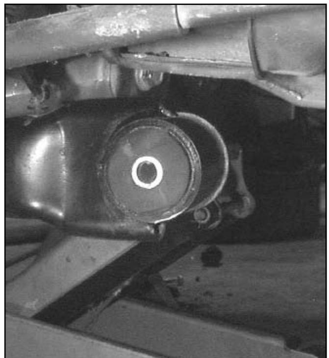
25. Raise the front of the IRS subframe into position and re-install the two front 12mm subframe mounting bolts. If the car is equipped with conventional rear coil springs, make sure they are positioned properly on the spring perches as the front of the IRS subframe is lifted into place.
