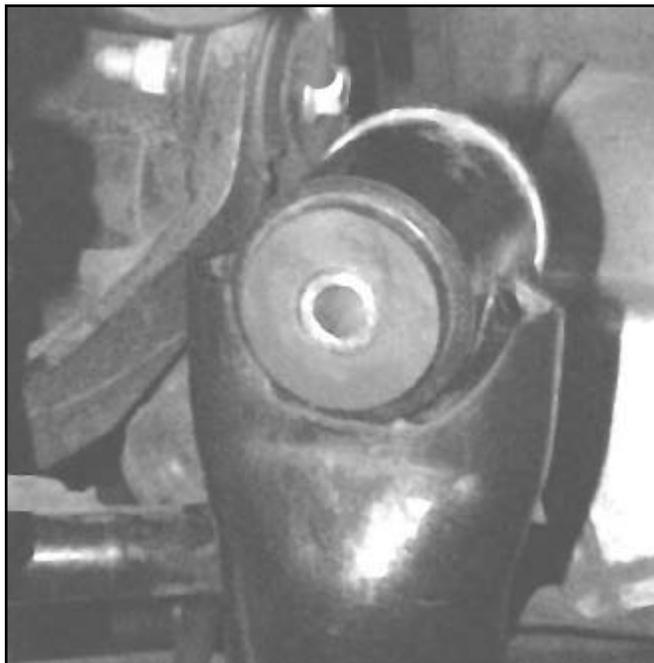
*Do NOT re-attach the rear of the IRS subframe to the chassis yet. You need to leave the rear of the IRS subframe on the jackstands to have sufficient clearance around the fuel tank to lower the front of the IRS subframe.*
