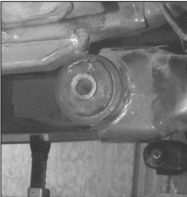
*NOTE: If you have an MMT-6 Bushing Removal Tool, remove the two front rubber bushings with the tool now. If you do not have the tool, use the procedure detailed in Step 9 to remove the rubber bushings.*
