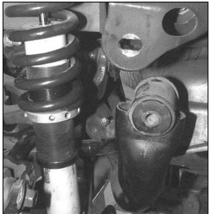
*NOTE: If you have an MMT-6 Bushing Removal Tool, remove the two rear rubber bushings with the tool now. If you do not have the tool, use the procedure detailed in Step 9 to remove the rubber bushings.*
