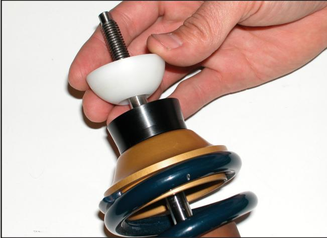
You have now completed one coil-over assembly. Repeat Steps 18 through 31 for the second shock.
