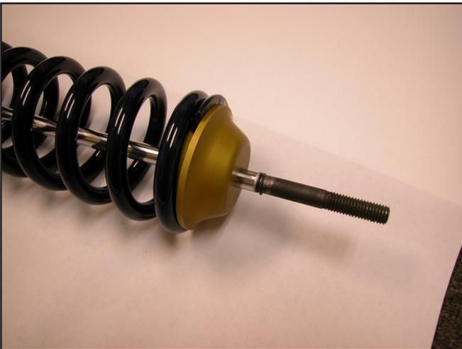
29. Place one of the aluminum pivot sockets on the shock shaft with the cup facing upward. The counterbore on the bottom side of the pivot socket will encapsulate the circlip.
