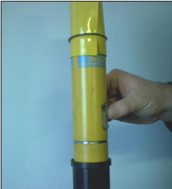
21. Grab the plastic sheet from the bottom with both hands. Slide it and the Spirolock ring over the shock body. Keep pulling until the Spirolock is close to the groove, then pull the plastic sheet out from under the Spirolock ring. Slide the Spirolock to the groove and let it snap into place within the groove.
