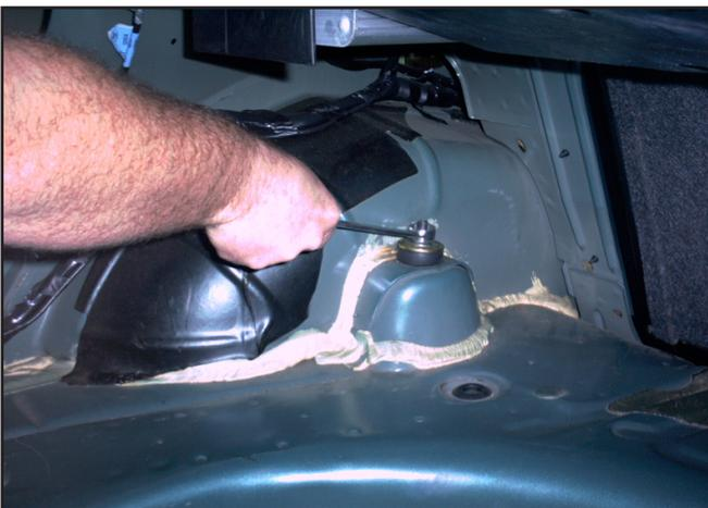
36. Raise the lower spring perch until the spring is just contacting the upper and lower spring perches.
