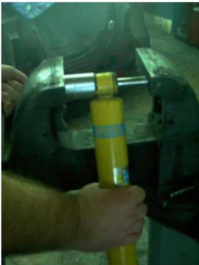
11. Use a similar process to remove the rubber bushings from each shock eyelet. Select a socket that is large enough to accept the rubber bushing into its center, but will still support the steel eye of the lower shock mount. Then select a smaller deep socket that will be able to push the rubber bushing out of the steel eye.
