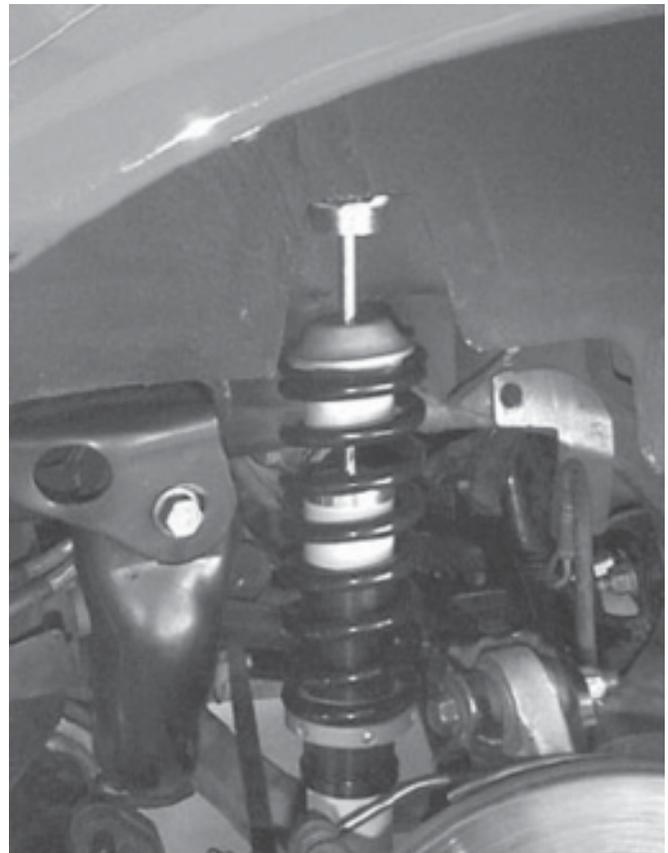
31. Completely coat the exposed faces of the urethane with the supplied grease.
