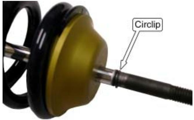
25. Observe the circlips provided. They are a stamping, therefore one side has sharp corners and one side has rounded corners. The side of the circlip with the sharp corners will be installed facing downward toward the spring perch.
