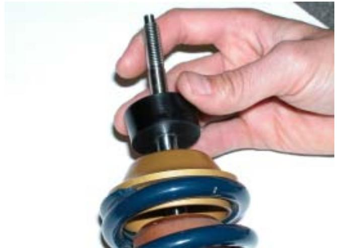
26. Orient the circlip with the sharp corners facing down toward the spring perch. Carefully thread the circlip down the threaded portion of the shaft until the threads stop. Carefully use a flat-blade screw driver to ease the circlip past the unthreaded portion of the shaft, sliding it down into the groove above the larger diameter portion of the shaft. The circlip should be tight around the shock shaft.
