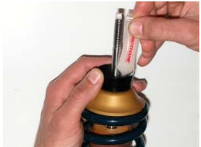
29. Place one of the Delrin pivot balls on the shock shaft with the curved side facing down toward the aluminum pivot socket.
