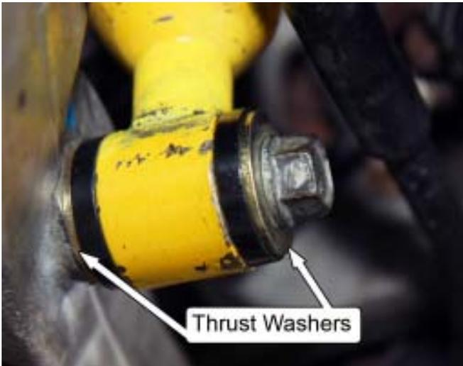
34. Thread the OEM 14mm bolt into the OEM special nut on the back side of the control arm. Torque the OEM 14mm lower shock bolt to 98ft-lb.
