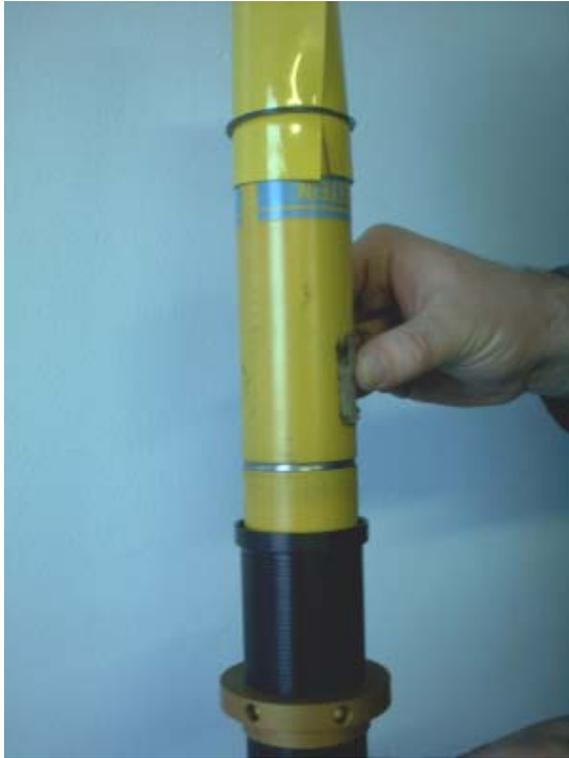
17. Grab the shim stock from the bottom with both hands. Slide it and the Spirolock ring over the shock body. Keep pulling until the Spirolock ring is close to the groove, then pull the shim stock out from under the Spirolock ring. Slide the Spirolock ring to the groove and let it snap into place within the groove.
