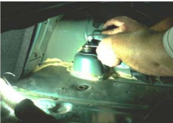
37. Raise the lower spring perch by threading it upwards until the spring is just contacting the upper and lower spring perches.
