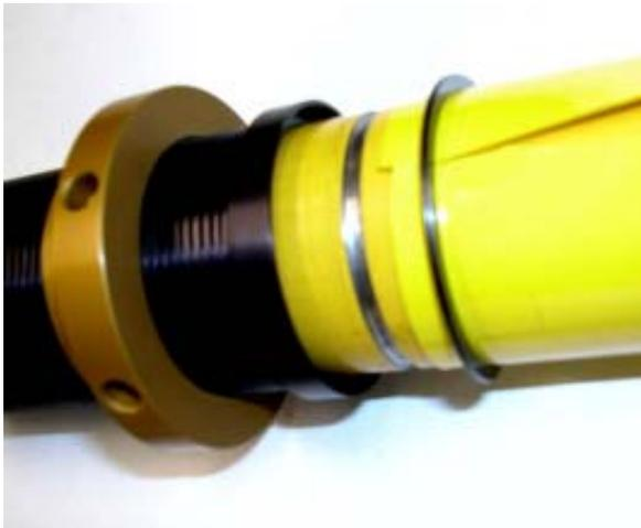
18. Slide the threaded sleeve down until it seats on the Spirolock ring.
