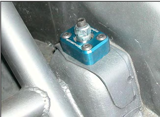
If you are using the Koni rod-end, install the rod-end in the clevis and tighten to manufacturer's specification.
