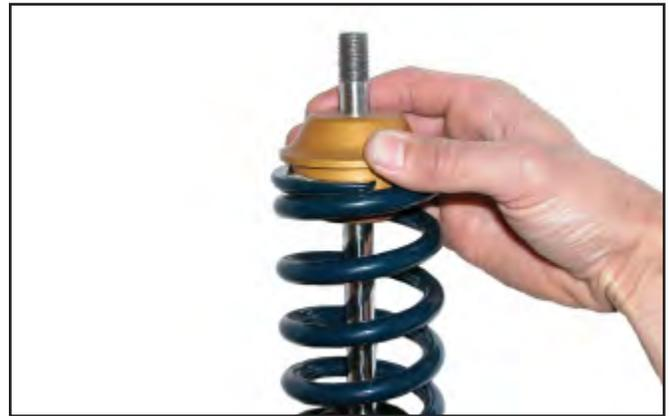
18. Thread the 14mm jam nut onto each shock until it bottoms against the smooth portion of the shaft. Do not force the nut once it has bottomed, as this will damage the threads.
