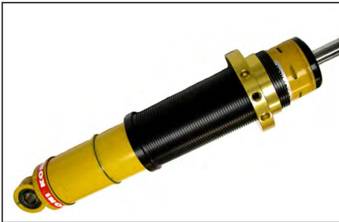
15. Place a 2-1/4" diameter coil-over spring onto each lower spring perch. Position the lower spring perch so the top of the spring is about 3" below the threaded portion of the shock shaft. This will make the installation of the rest of the parts easier.
