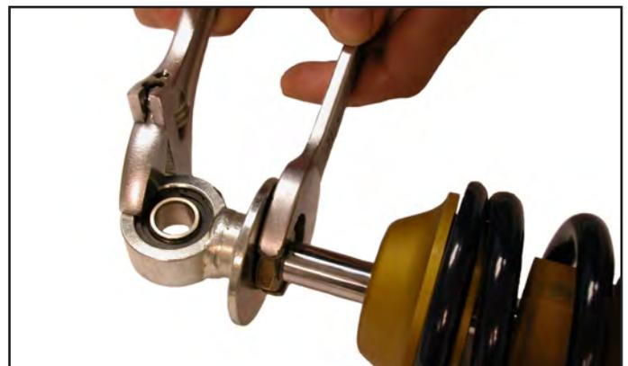
20. Insert two bearing inserts into the lower rod-end of the shock.
