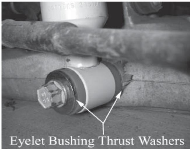
26. Thread the OEM 14mm bolt into the OEM special nut on the back side of the control arm. Torque the OEM 14mm lower shock bolt to 98ft-lb.
