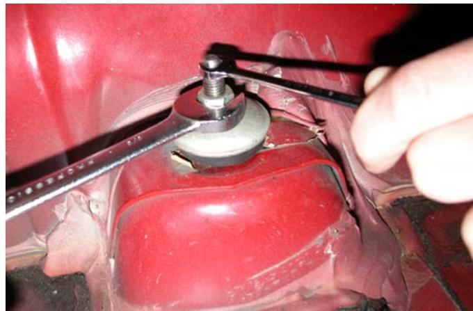
29. Raise the lower spring perch until the spring is just contacting the upper and lower spring perches.
