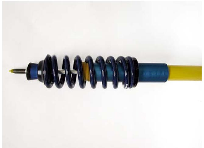
23. On the passenger side of the car, position the shock shaft of one of the completed coil-over assemblies through the hole in the shock tower.
