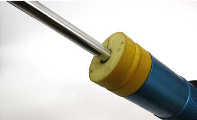
16. Lube two of the MM lower shock mount urethane bushings, inside and out, with the supplied grease. Completely coat the bare metal surfaces inside the shock eyelet with grease. Then, push the greased urethane bushings into the eyelet of the shock.
