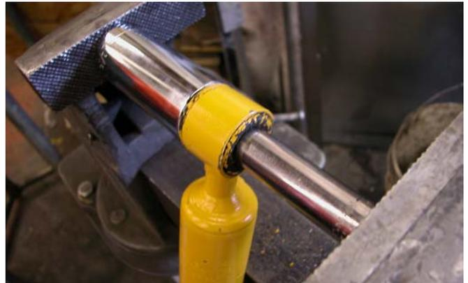
10. Use a similar process to remove the rubber bushings from each shock eyelet. Select a socket that is large enough to accept the rubber bushing into its center, but will still support the steel eye of the lower shock mount. Then select a smaller deep socket that will be able to push the rubber bushing out of the steel eye.
