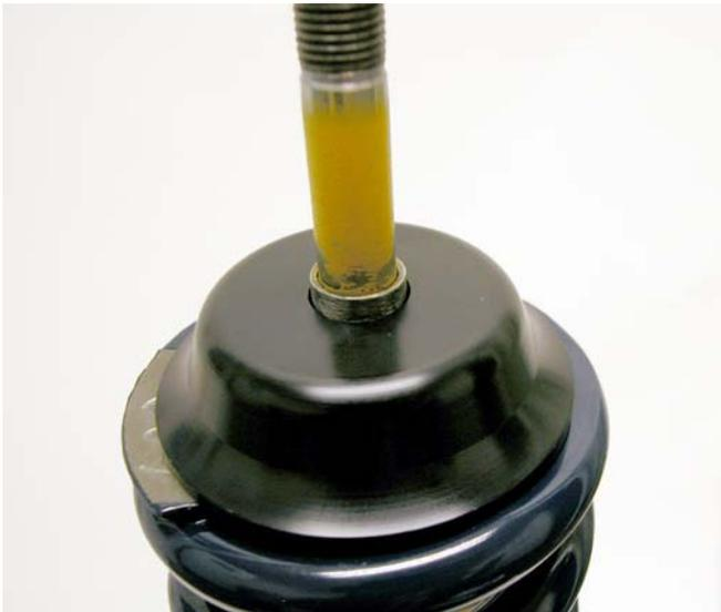
20. Place one of the aluminum pivot sockets over the piston rod (with the cup facing upward) until it seats against the welded isolator bung located near the top of the shock piston rod.
