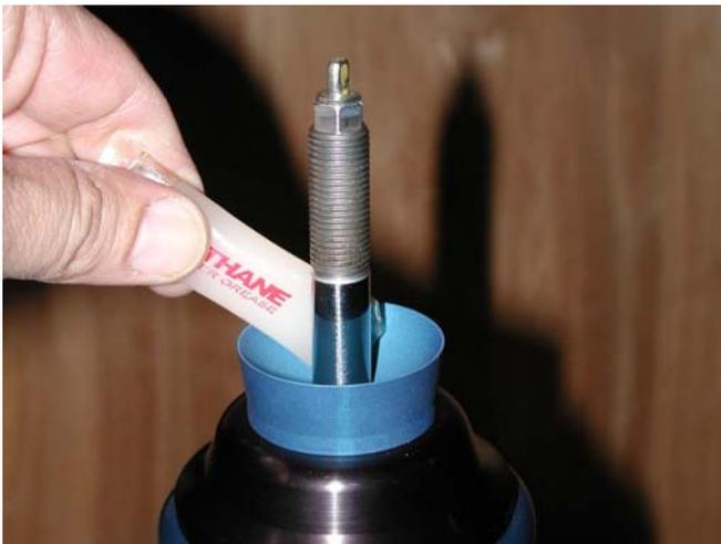
22. Place one of the Delrin pivot balls on the shock shaft with the curved side facing down toward the aluminum pivot socket.
