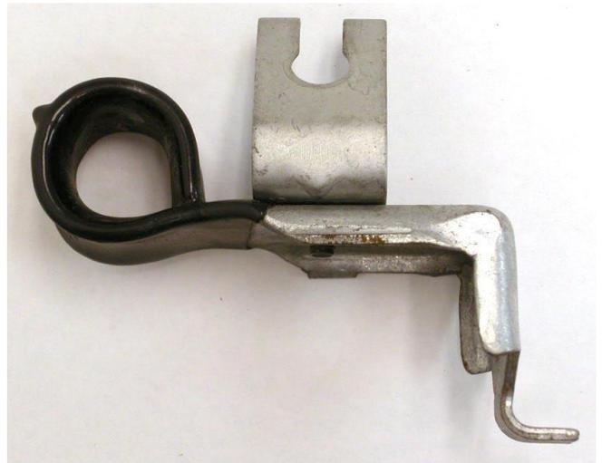
15. Slide the bracket back onto the parking brake cable and reattach the parking brake cable to the caliper.
