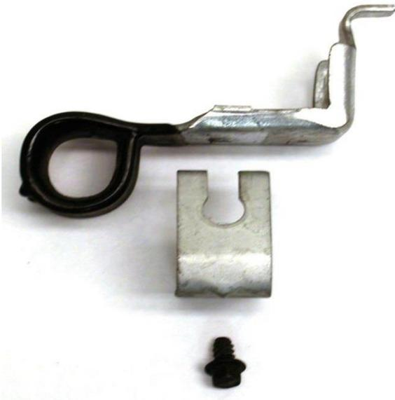
12. Flip the parking brake bracket 180 degrees and place the ABS bracket on top of the parking brake bracket.
