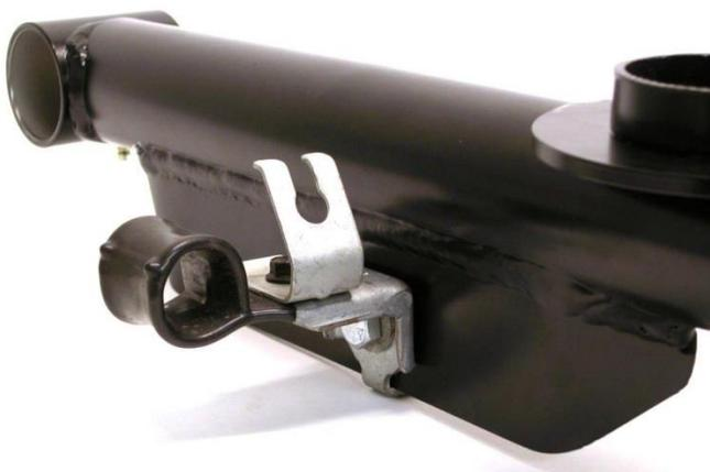
27. Reattach the ABS wires on both sides of the car.
