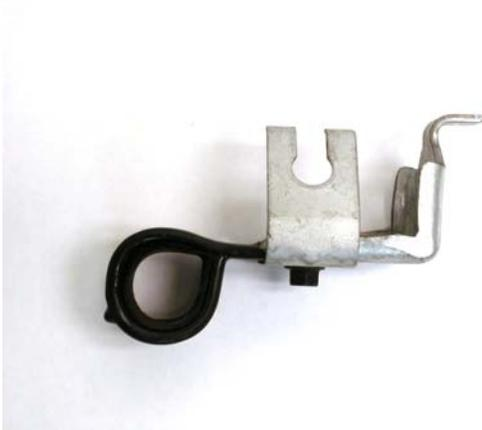
13. Flip the Parking Brake Cable Bracket 180 degrees and place the ABS Bracket on top of the Parking Brake Cable Bracket.
