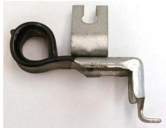
15. Slide the Parking Brake Cable Bracket back onto the parking brake cable and reattach the parking brake cable to the caliper.
