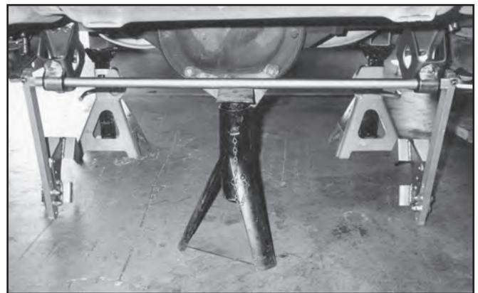
24. Mate the Axle Mounts to the axle; their exact position at this time is not critical. As you do so, slide a U-bolt into place on each Axle Mount. Be careful to not pinch the brake lines. Thread (8) 3/8" Nylock Nuts onto the U-Bolts, placing one 3/8" Grade 8 washer under each nut. Leave the brackets slightly loose so they can pivot on the axle tubes. **NEVER** weld the Axle Mounts to the axle! Welding on the axle will cause the axle to warp!
