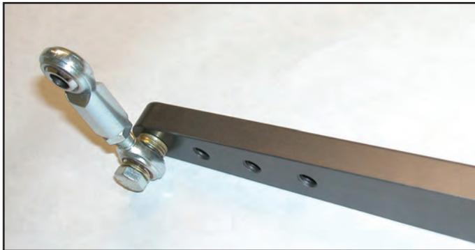
62. On the opposite side of the car, adjust the length of the Rod-end assembly so that the 3/8" X 1 1/2" G5 mounting bolt easily slides through the Male Rod-end and the mounting hole in the Swaybar Arm. This procedure ensures the Swaybar is not preloaded. Assemble the hardware as in Step 61, and torque the bolt to 33 ft-lb.
