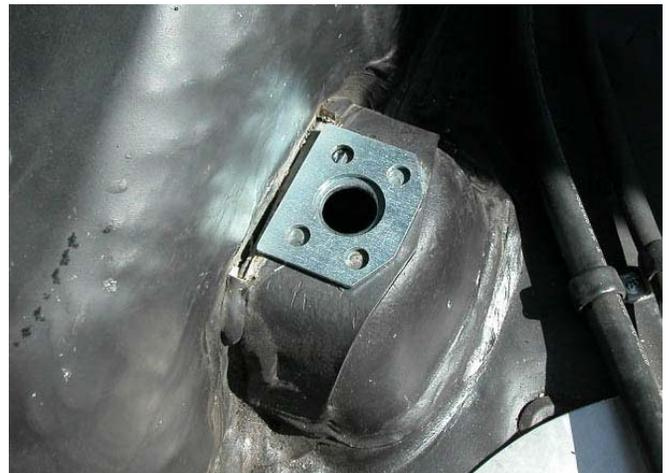
8. Mark the position of the four mounting holes onto the shock tower. Remove the Doubler Plate. Center punch the location of the hole centers. Drill four 1/8" pilot holes. Drill to the final size of 11/32". Deburr the holes.
