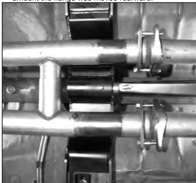
31. Raise the H-pipe and transmission exhaust hanger back into place. Re-attach the transmission mount to the transmission.
