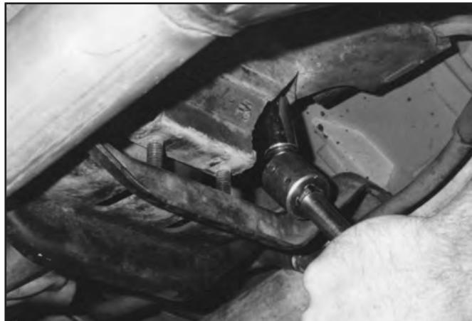
32. Bolt the transmission crossmember to the transmission mount. Slide the bolts between the transmission crossmember and the chassis in place. Lower the floor-jack supporting the transmission.
