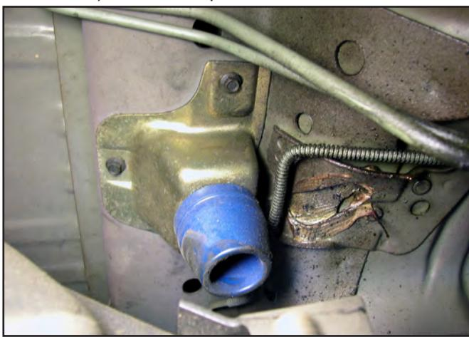
4. Clean and degrease the top and the bottom of the differential flanges where the vibration damper was bolted (typically, there is a lot of caked on dirt and grease). These flanges must be clean before attaching the TA.
