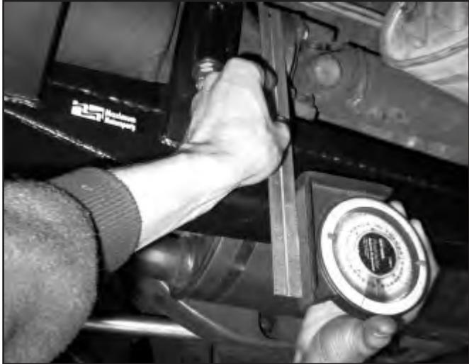
39. Measure the transmission output shaft angle. The easiest way to do this is to place the angle finder on the front of the crank pulley.
