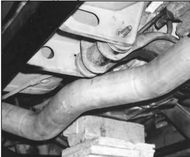
33. Check the clearance between the exhaust pipes and the TA Crossmember.
