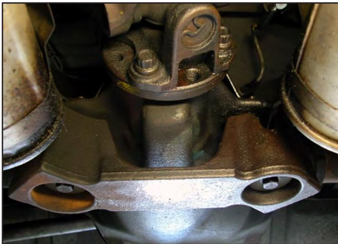
3. Remove the pinion snubber assembly from the bottom of the chassis (directly above the front of the differential). It is held in place with three small screws.
