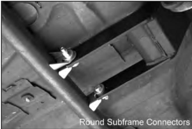
17. Mark the areas to be welded. Lower the TA and TA Crossmember and clean any paint or plating from the connectors in the area to be welded.
