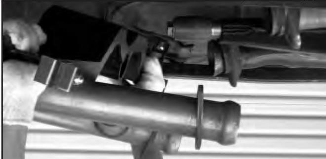
14. The TA Crossmember may now be slid rearwards while inserting the Urethane Pivot Bolt Assembly into the TA Crossmember Receiver Tube.
