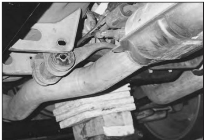
8. Lower and rotate the transmission crossmember to provide access to the two bolts holding the transmission mount to the transmission. Remove these bolts to allow the H-pipe to drop down away from the chassis during installation.
