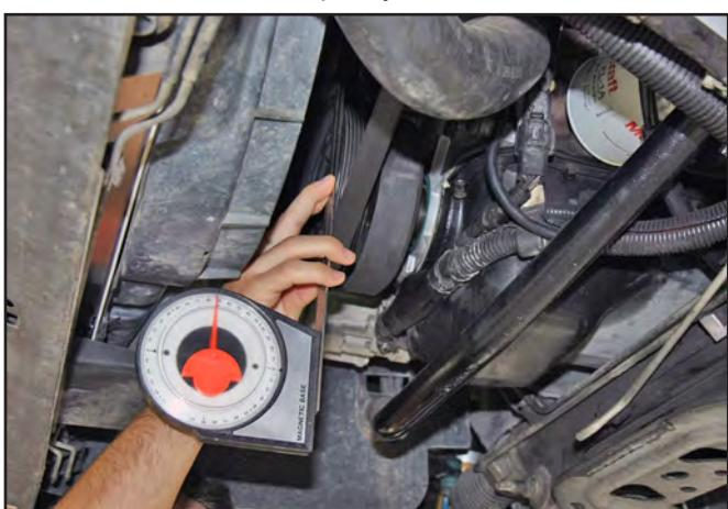
40. The goal is to make the pinion angle of the differential match the transmission output shaft angle. Each 2" shim will add or subtract 1/2 degree. Do not be surprised if you have to raise the front of the differ-
